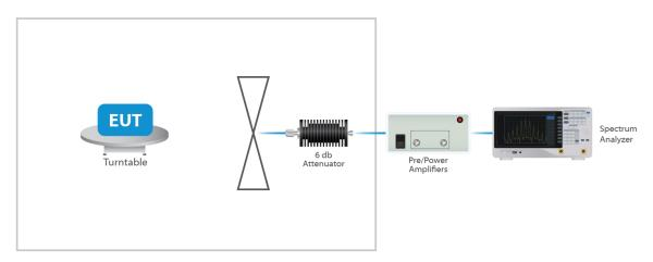
Figure 1: Radiated Emissions Test
