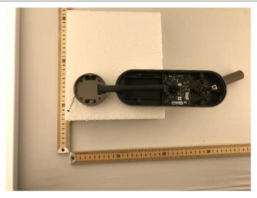
**Photograph 1: Connected Circuit Boards in Housing**
