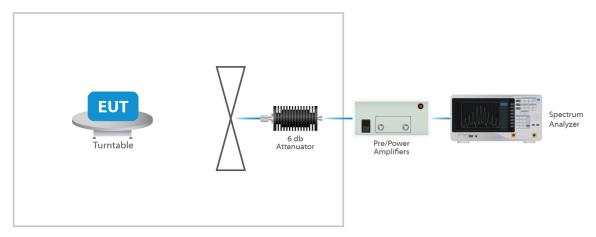
Figure 1: Radiated Emissions Test
