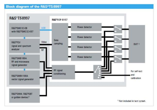
**Diagram 1: Test Configuration Block Diagram**
