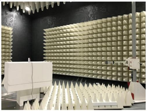
Photograph 2: Side View Test Set Up Radiated Emissions 1 – 17 GHz
