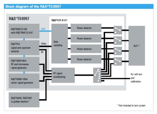
Diagram 1: Test Configuration Block Diagram
