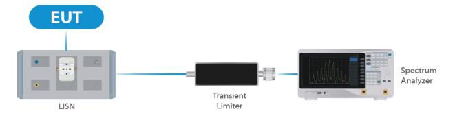
**Figure 1: Conducted Emissions Test**
