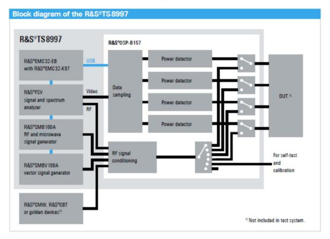
**Diagram 1: Test Configuration Block Diagram**
