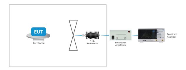
Figure 3: Radiated Emissions Test
