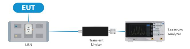
**Figure 1: Conducted Emissions Test**
