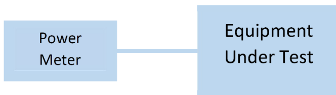
Figure 3: Output Power Measurement
