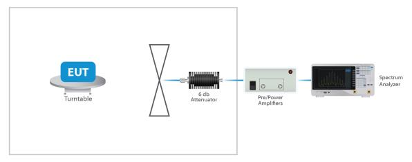
Figure 3: Radiated Emissions Test
