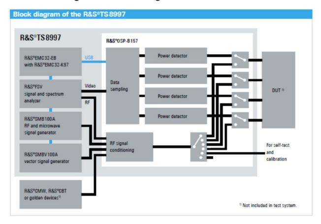
**Diagram 1: Test Configuration Block Diagram**
