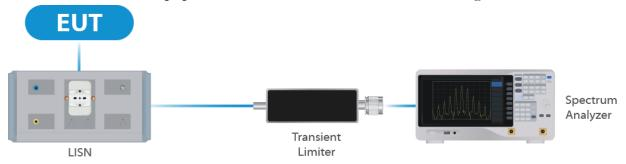
**Figure 1: Conducted Emissions Test**
