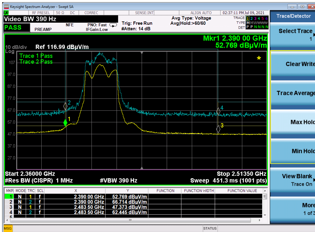
Graph 15: Lower Band Edge Plot – 2412 MHz – ax20 Mode
