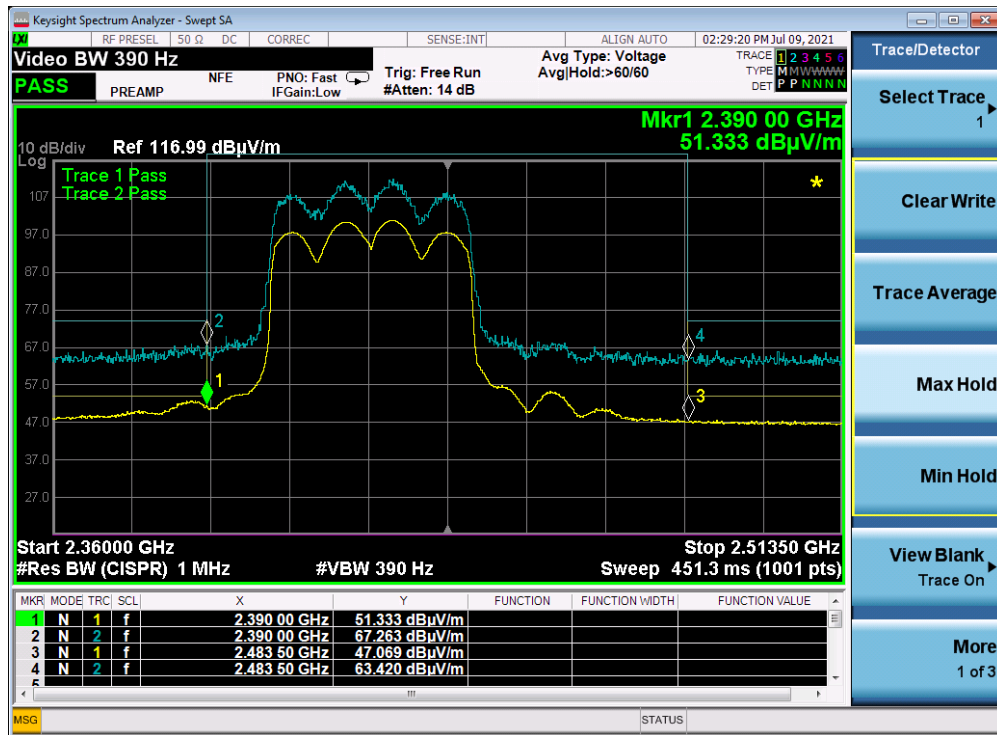
Graph 12: Lower Band Edge Plot – 2422 MHz – n40 Mode
