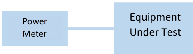
Figure 2: Direct Connect at the Antenna Port Test
