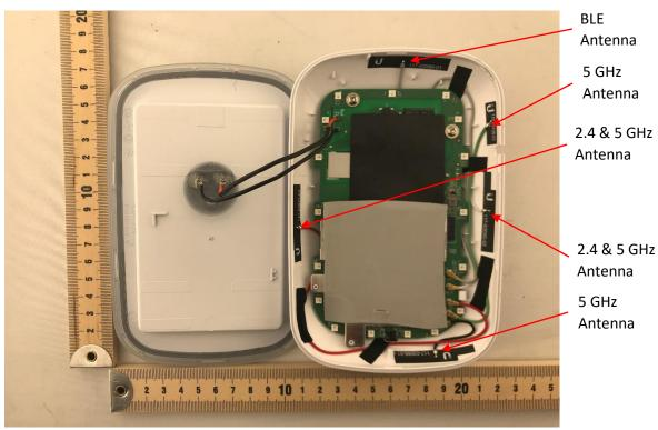
**Photograph 1: Back View of Circuit Board With Heat Sink**
