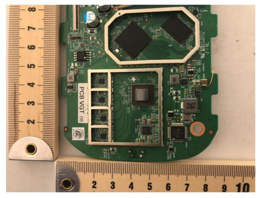
Photograph 5: Close Up View of Circuit Board RF Section
