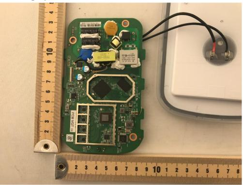
**Photograph 4: Front View of Circuit Board Without RF Cans**
