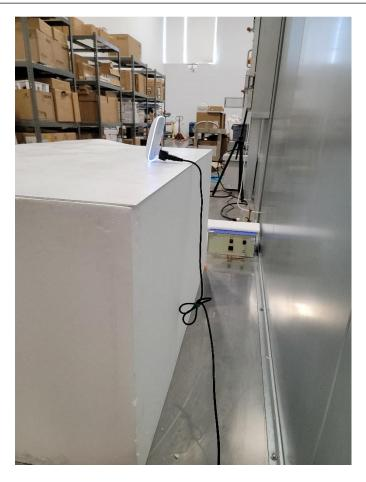
Photograph 5: Back Test Set Up AC Mains Conducted Emissions
