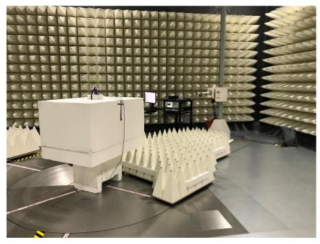
Photograph 3: Test Set Up Radiated Emissions 17 – 40 GHz
