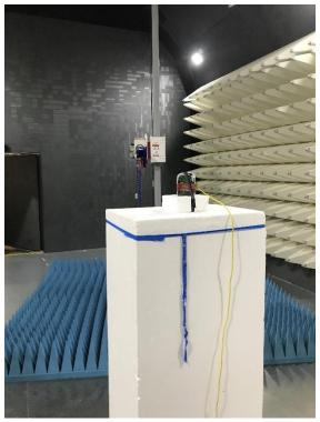
Photograph 2: Test Set Up Radiated Emissions 1 – 17 GHz
