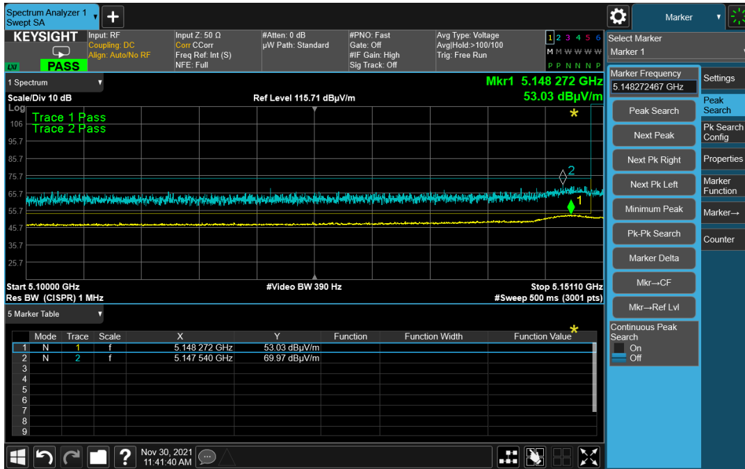
Graph 5: Radiated Lower Band Edge Plot – n Mode 40 MHz
