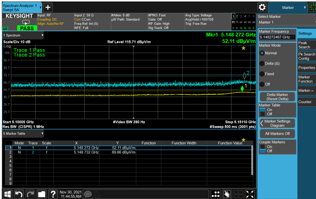
Graph 6: Radiated Upper Band Edge Plot – n Mode 40 MHz
