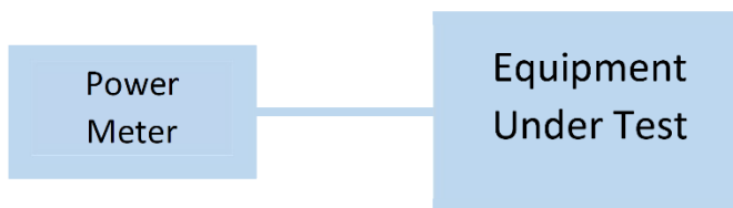
Figure 3: Output Power Measurement
