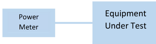
Figure 3: Output Power Measurement
