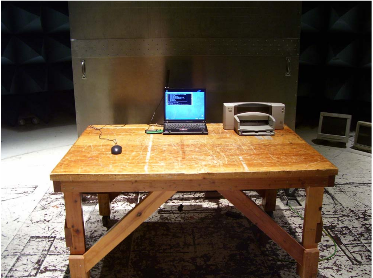
Photograph 2. Conducted Emissions Test Setup
