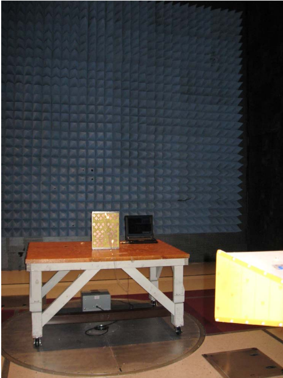
Photograph 5. Test Equipment and setup for various Radiated Measurements – 5.8GHz Panel Antenna
