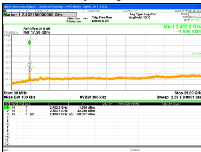
Chain0 : Conducted Spurious @ GFSK mode Ch Middle
