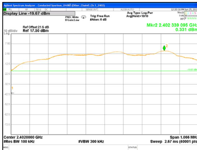
Chain0 : Conducted Spurious @ GFSK mode Ch Low
