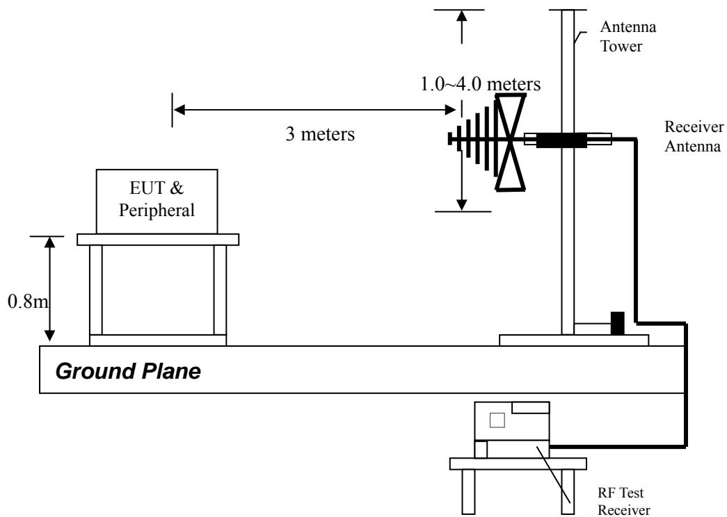
**7.5.3 Radiated emission above 1GHz using Horn Antenna**
