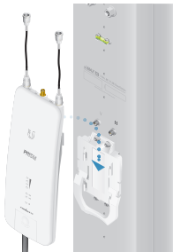
Mounting on a Sector Antenna
