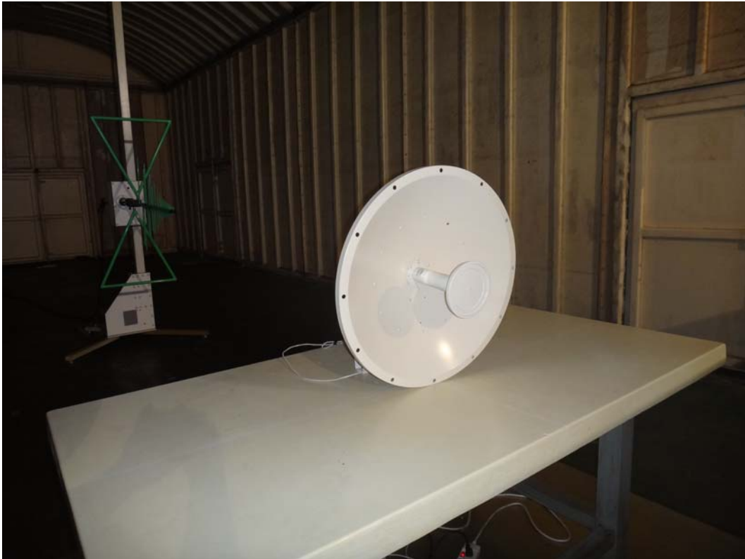
Back View of Radiated Test – Dish Antenna
