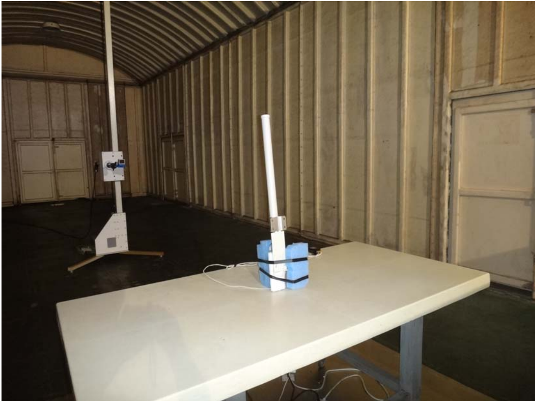
Back View of Radiated Test (Horn) - Omni Antenna
