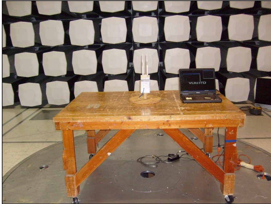
Photograph 3. Radiated Emission, Test Setup
