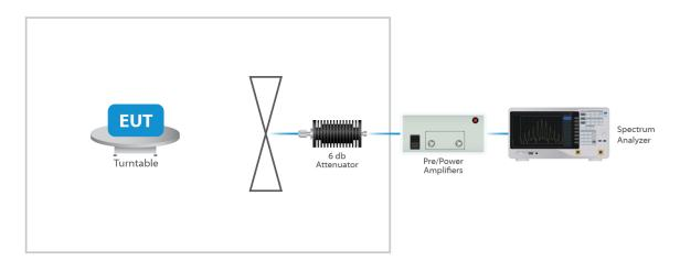
Figure 3: Radiated Emissions Test
