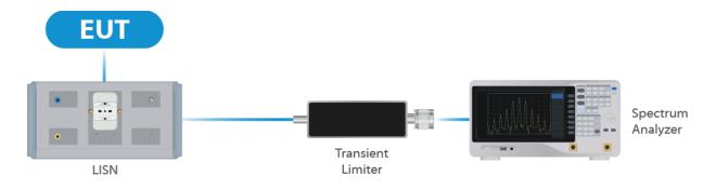
**Figure 1: Conducted Emissions Test**
