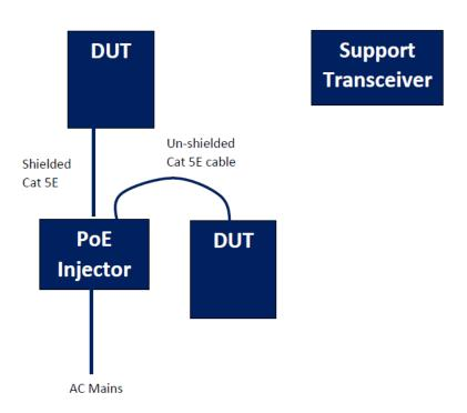
**Diagram 1: Test Configuration Block Diagram**
