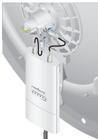
Connecting to a Dish Antenna
