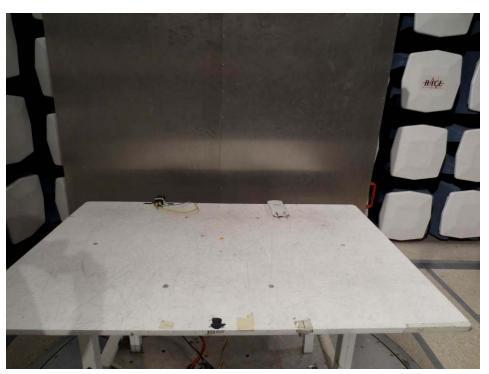
13.2 AC Line Conducted Emission Side View
