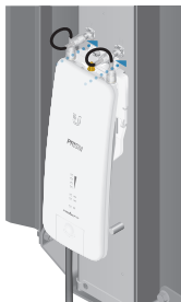
Connecting to a Sector Antenna
