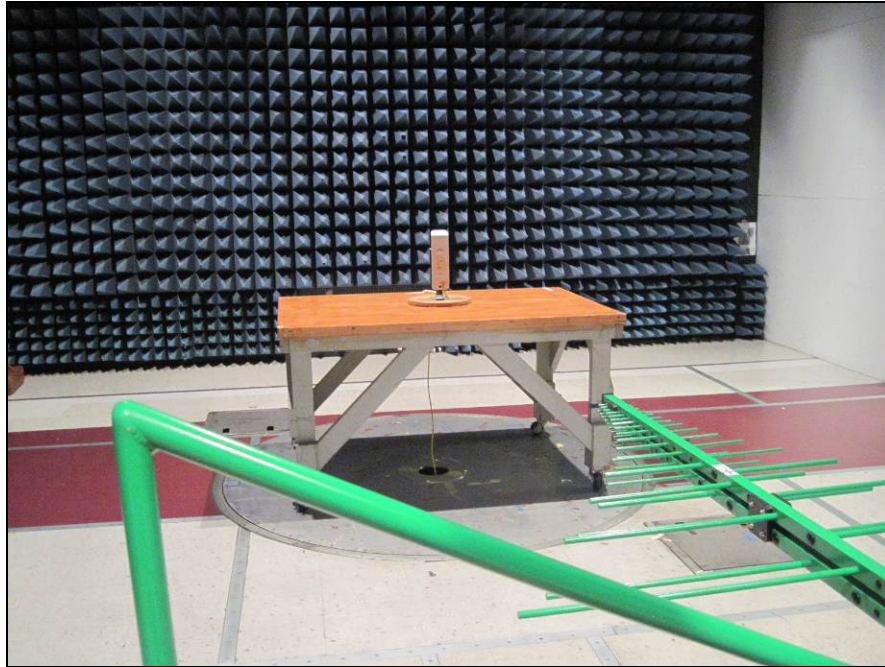
Photograph 6. Radiated Spurious Emissions, Test Setup, 30 MHz – 1 GHz
