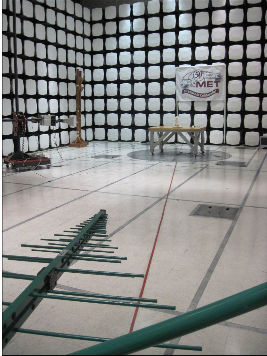
Photograph 4. Radiated Emission, Test Setup
