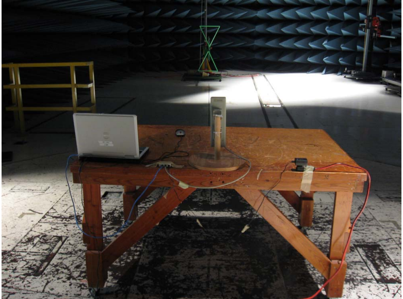
Photograph 2. Radiated Emission Test Setup 30 MHz - 2 GHz
