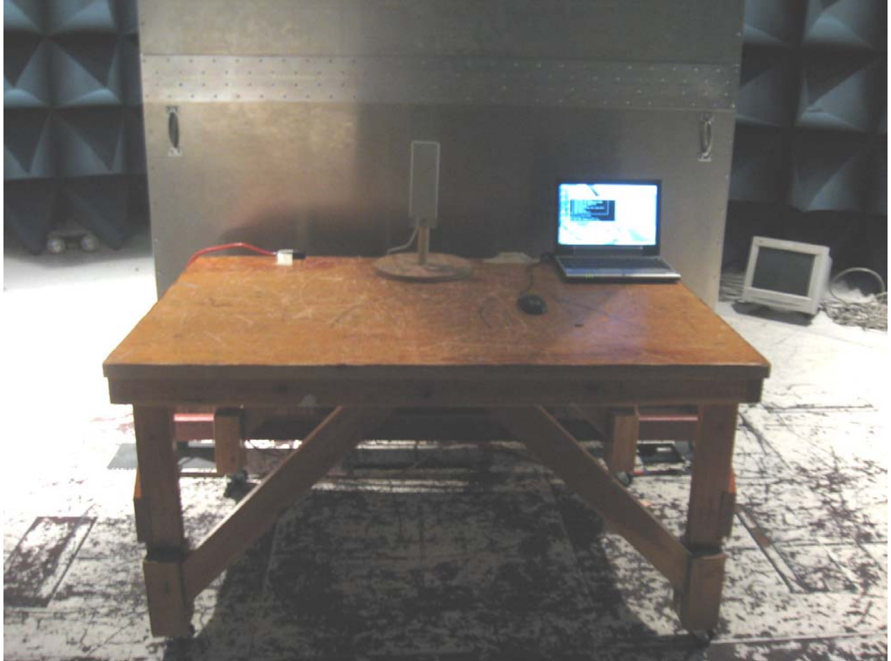
Photograph 1. Conducted Emissions Test Setup
