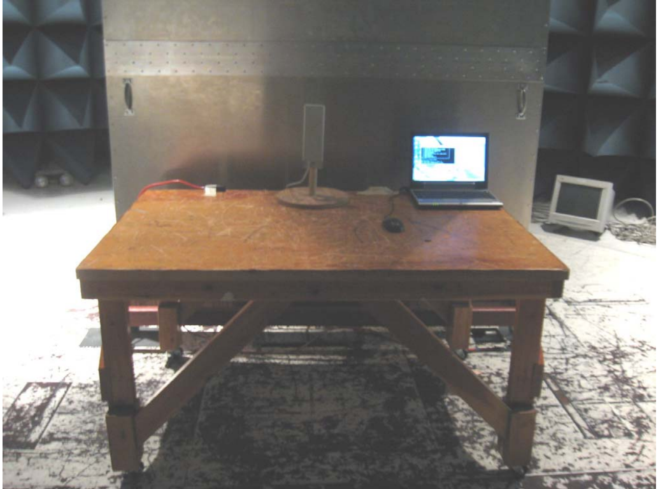
Photograph 2. Conducted Emissions Test Setup
