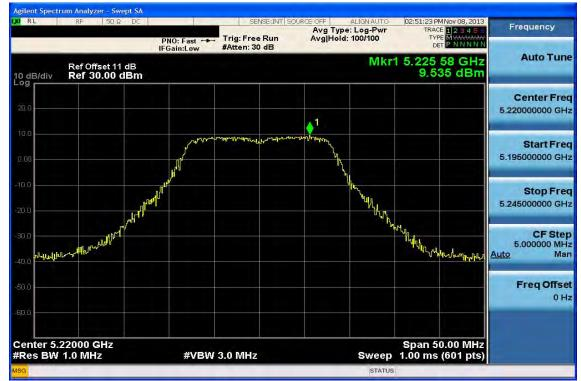
802.11n HT20, 5150~5250 MHz, Peak Value Data Plot (CH Mid 5220 MHz)
