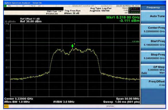
802.11n HT20, 5150~5250 MHz, PPSD Data Plot (CH Mid 5220 MHz)
