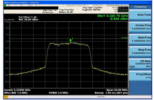
802.11n HT20, 5150~5250 MHz, PPSD Data Plot (CH Mid 5220 MHz)
