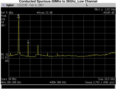
Conducted Spurious-30Mhz to 26Ghz\_Low Channel
