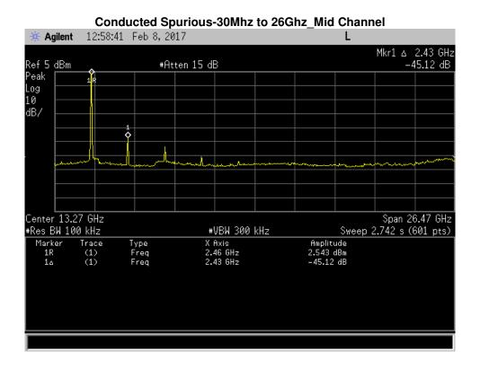
The below plot is to show the output power of the device remains compliant when measuring peak power. The 20dBc test results are in reference to this fact.
