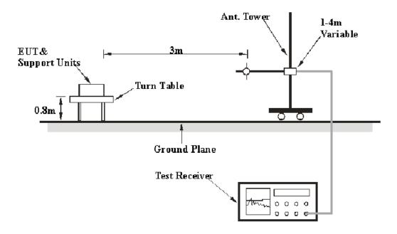
The radiated emission and out of band emission tests were performed in the 3 meters chamber test site, using the setup accordance with the ANSI C63.4-2009. The specification used was the FCC 15.209 /205and FCC 15.245 limits.
