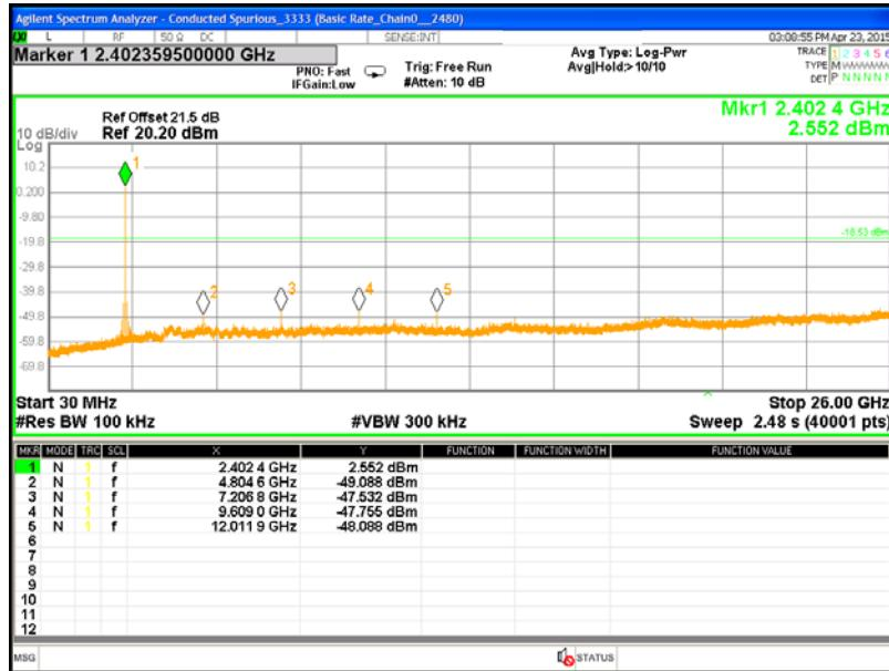
Conducted Spurious @ GFSK mode ch20 (30M-26G)
