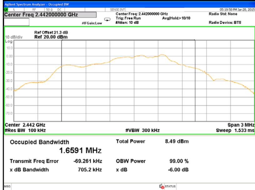
6dB Occupied Bandwidth @ GFSK mode Ch High
