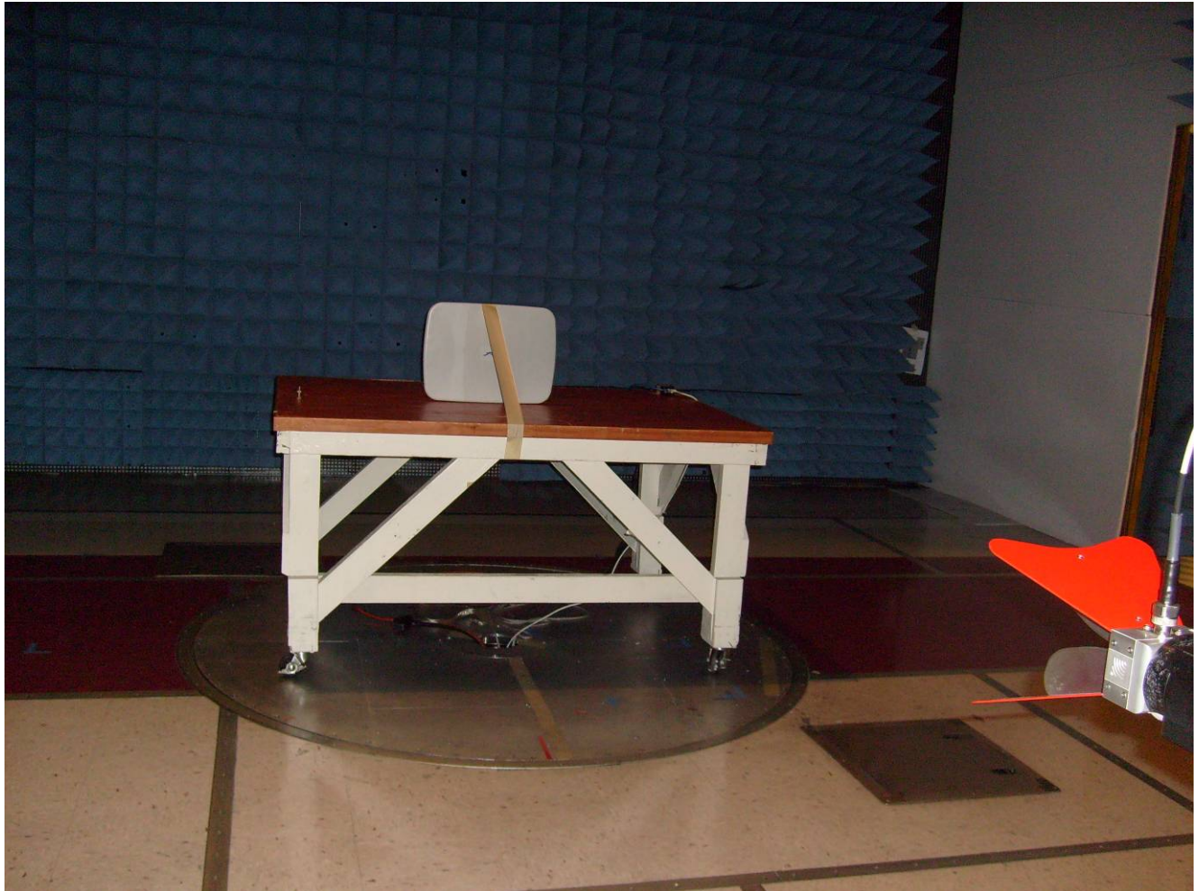
Photograph 5. Radiated Emission, above 1GHz Test Setup
