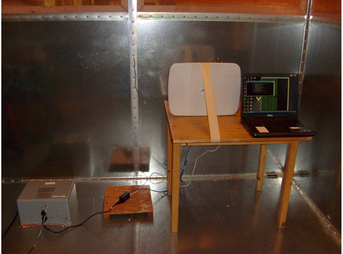
Photograph 6. Conducted Emissions, 15.207, Test Setup
