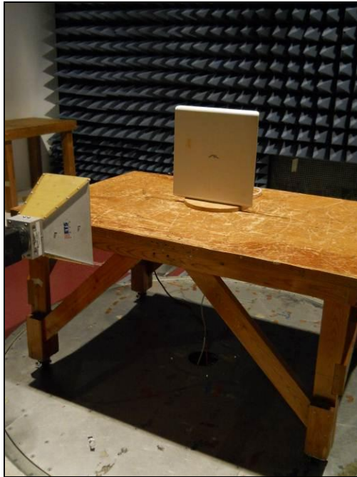
Photograph 6. Radiated Spurious Emissions, Test Setup, 1 GHz – 18 GHz
