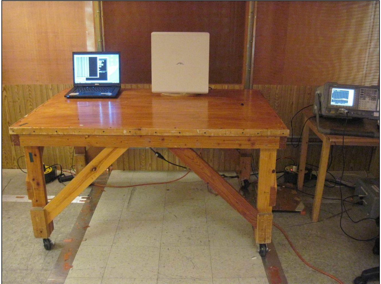
Photograph 2. Conducted Emissions, Test Setup
