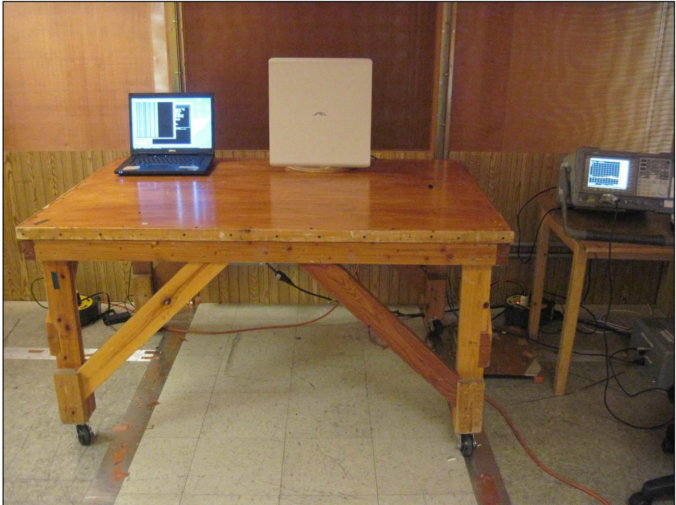
Photograph 4. Conducted Emissions, 15.207(a), Test Setup
