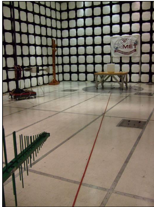
Photograph 6. Radiated Spurious Emissions, Test Setup, 30 MHz – 1 GHz
