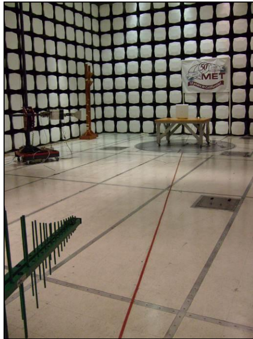
Photograph 6. Radiated Spurious Emissions, Test Setup, 30 MHz – 1 GHz
