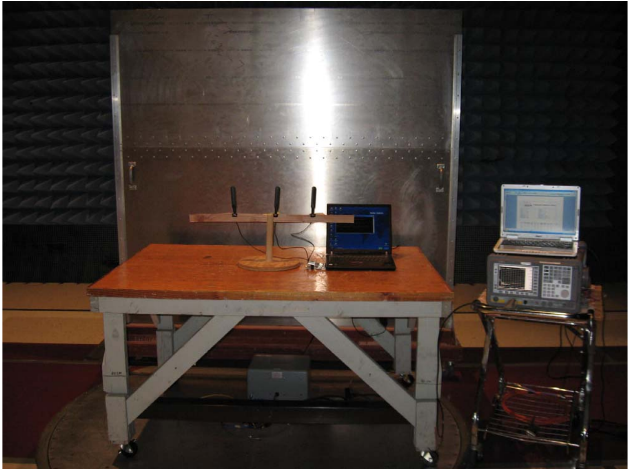
Photograph 2. Conducted Emissions Test Setup
