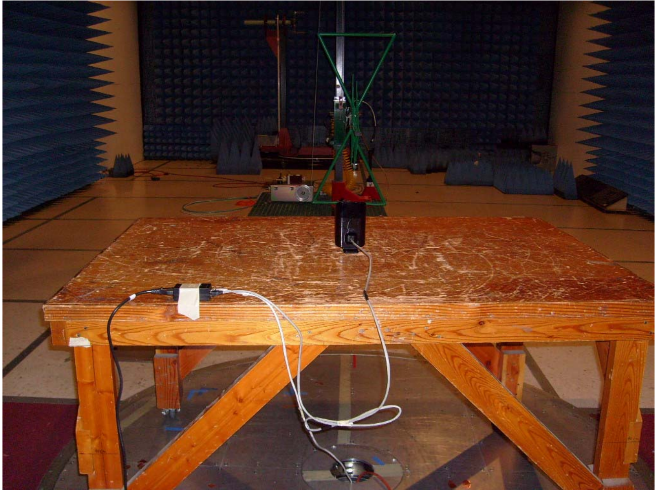
Photograph 3. Radiated Emission, 30MHz – 1GHz Test Setup (Back View)
