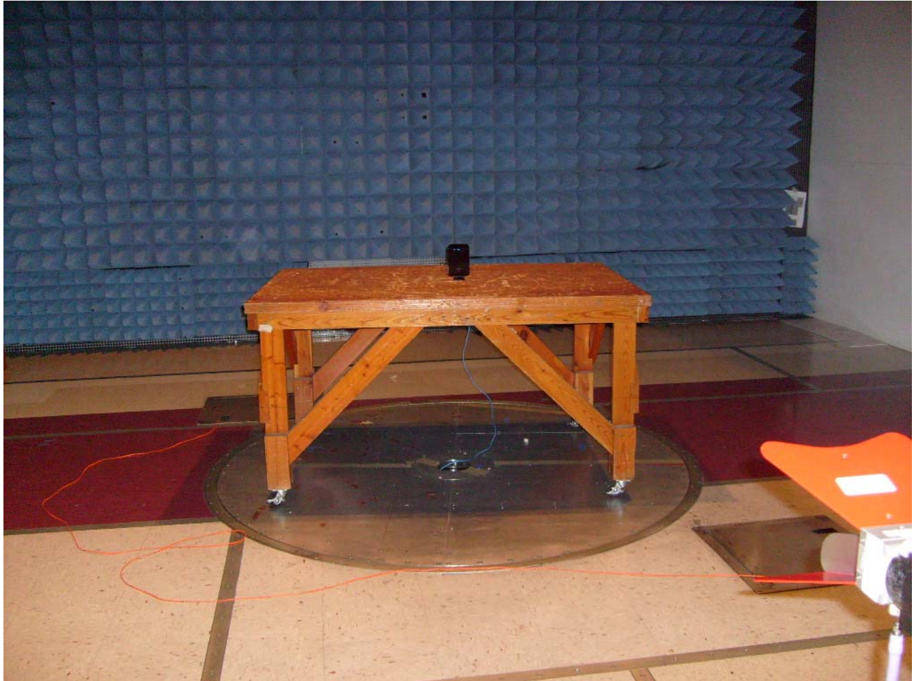
Photograph 4. Radiated Emission, above 1GHz Test Setup
