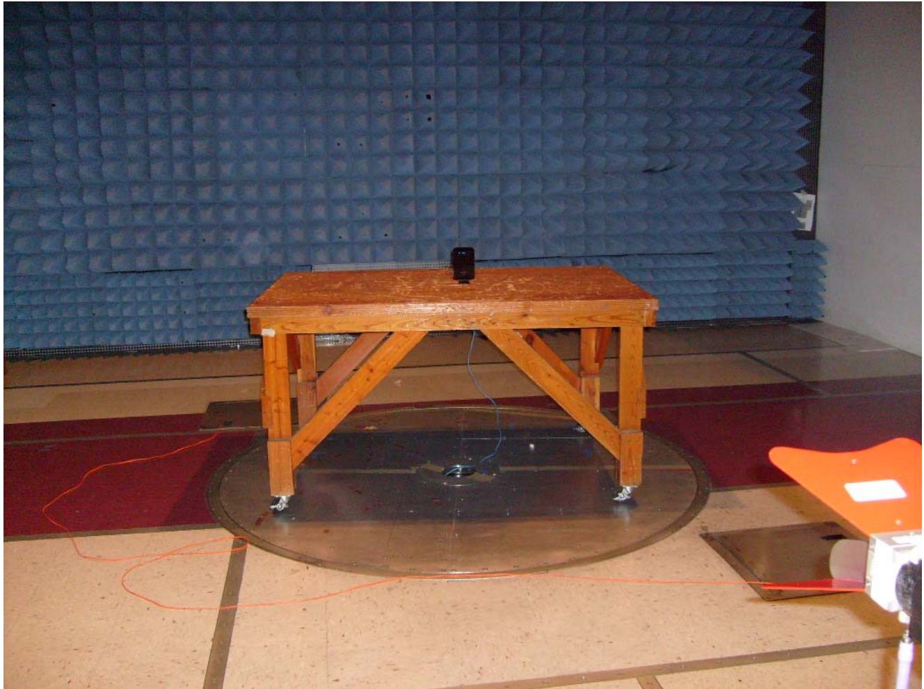
Photograph 6. Radiated Spurious Emission, Test Setup, 3m Distance
