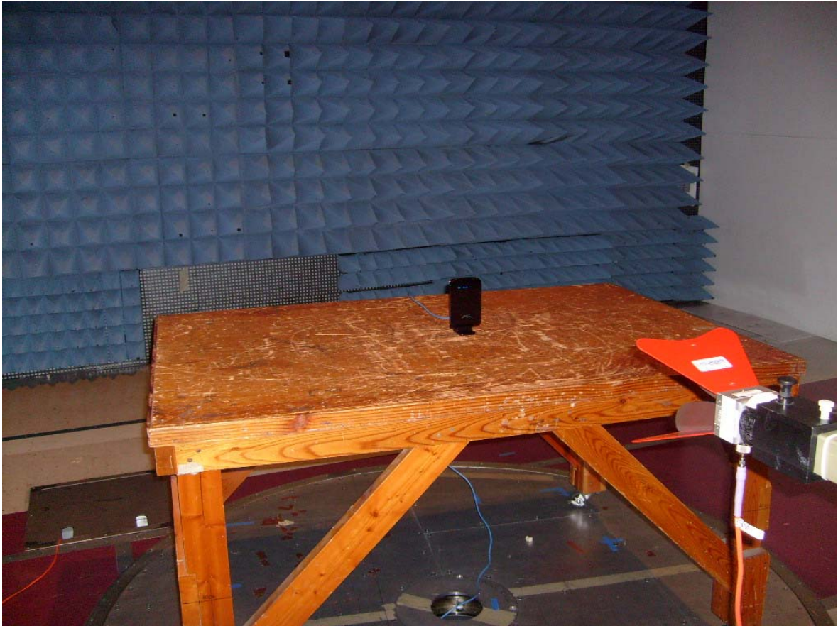
Photograph 7. Radiated Spurious Emission, Test Setup, 1m Distance
