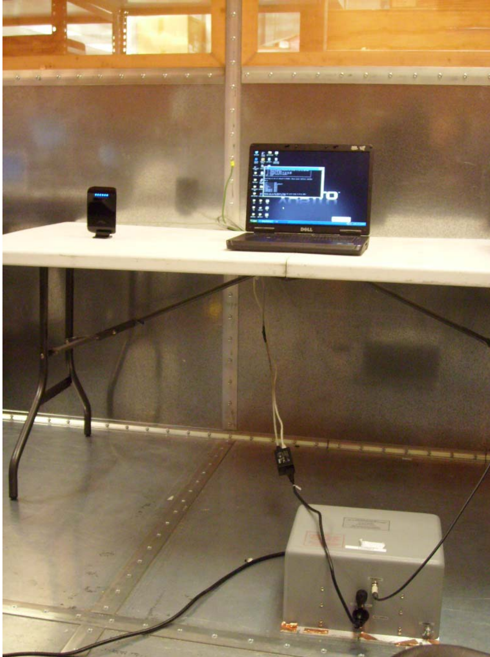
Photograph 5. Conducted Emissions, 15.207, Test Setup
