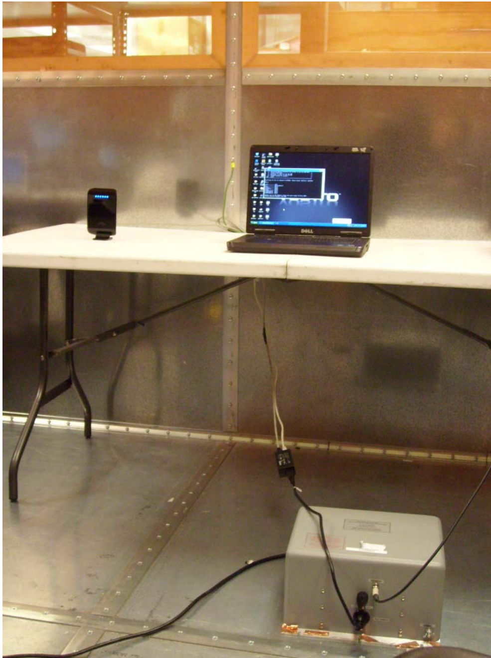
Photograph 1. Conducted Emissions, Test Setup
