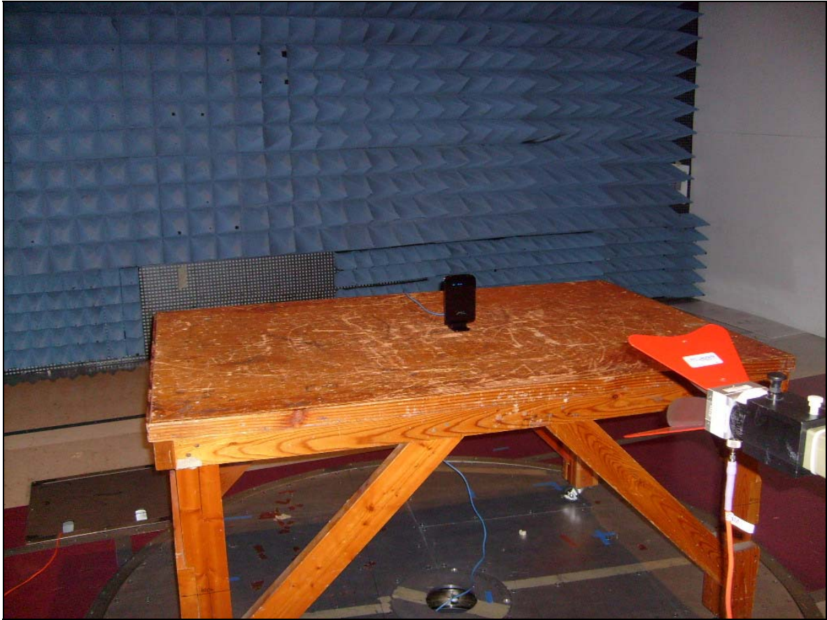
Photograph 7. Radiated Spurious Emission, Test Setup, 1m Distance
