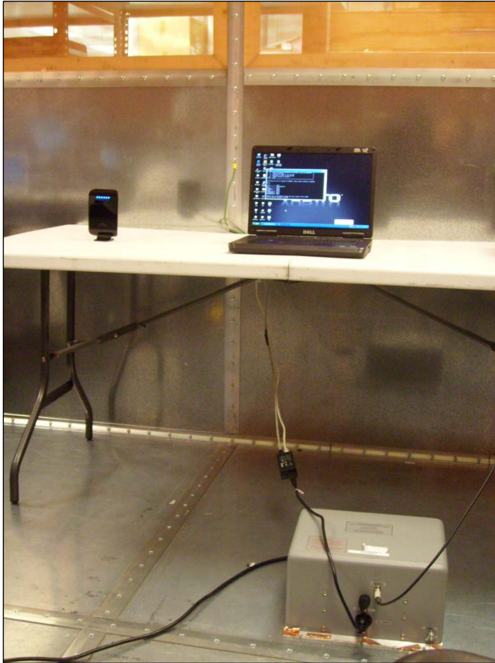
Photograph 5. Conducted Emissions, 15.207, Test Setup
