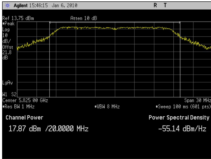
Plot 40. Peak Output Power 5825MHz High Channel 802.11n 20MHz Port 2
