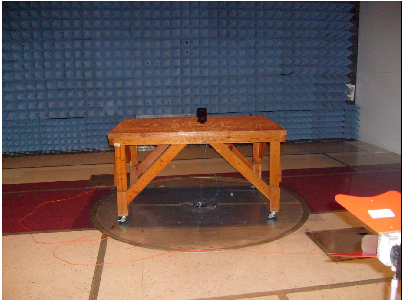
Photograph 6. Radiated Spurious Emission, Test Setup, 3m Distance
