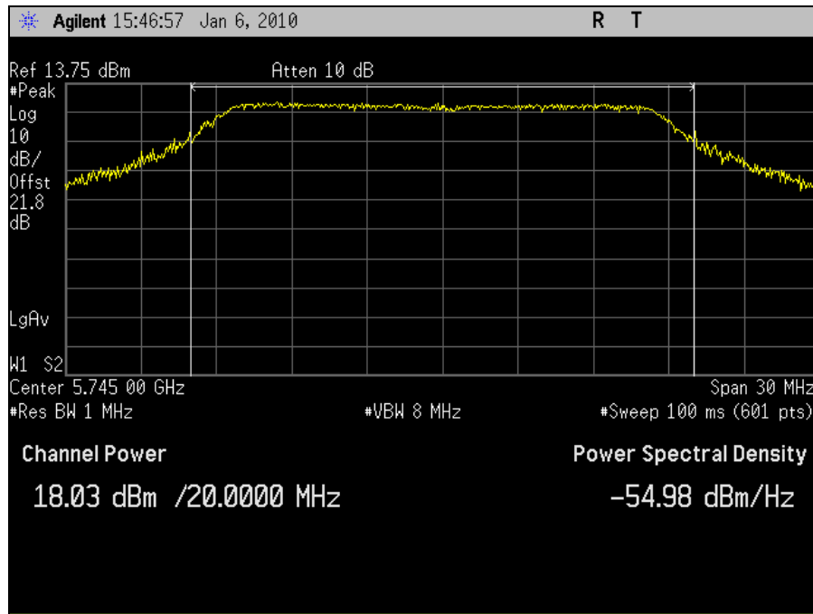
Plot 38. Peak Output Power 5745MHz Low Channel 802.11n 20MHz Port 2
