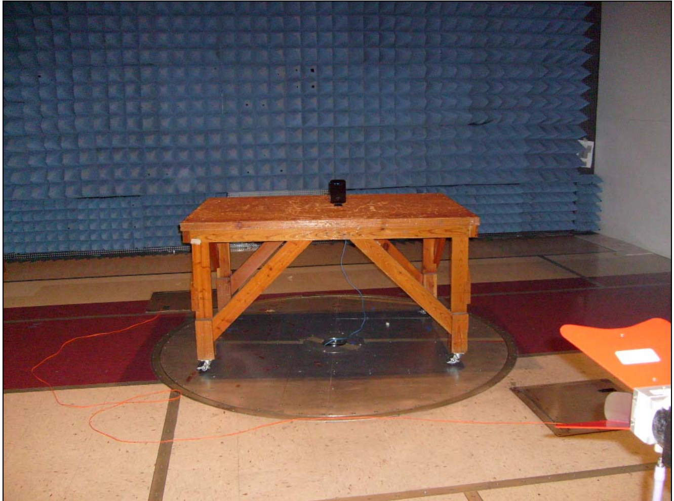
Photograph 4. Radiated Emission, above 1GHz Test Setup
