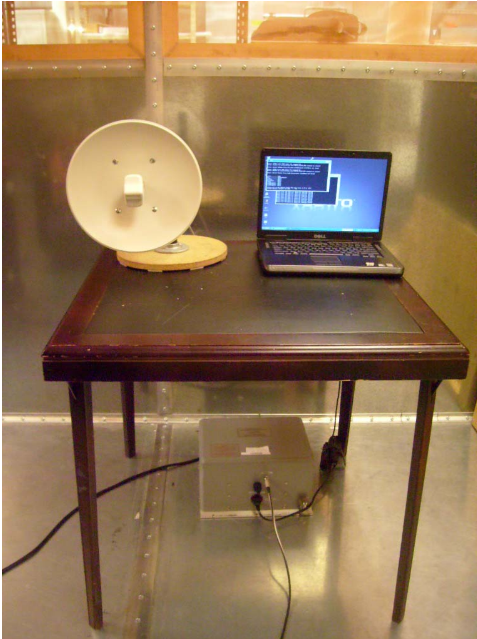
Photograph 4. Conducted Emissions, 15.207, Test Setup
