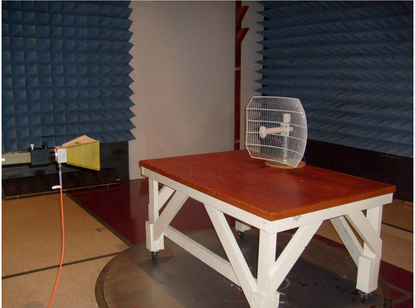
Photograph 6. Radiated Spurious, Test Setup (Grid Antenna)
