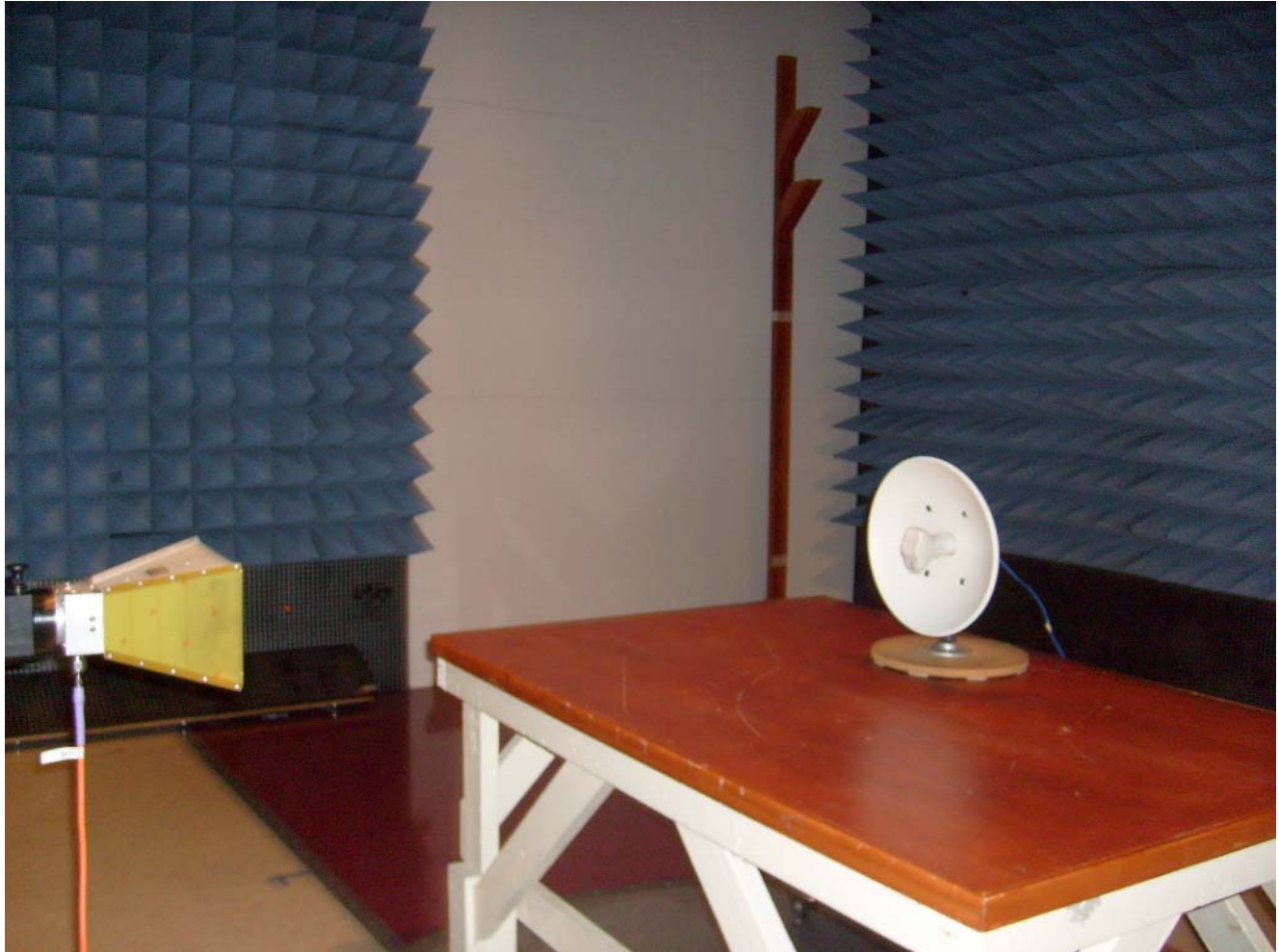
Photograph 5. Radiated Spurious, Test Setup (Dish Antenna)
