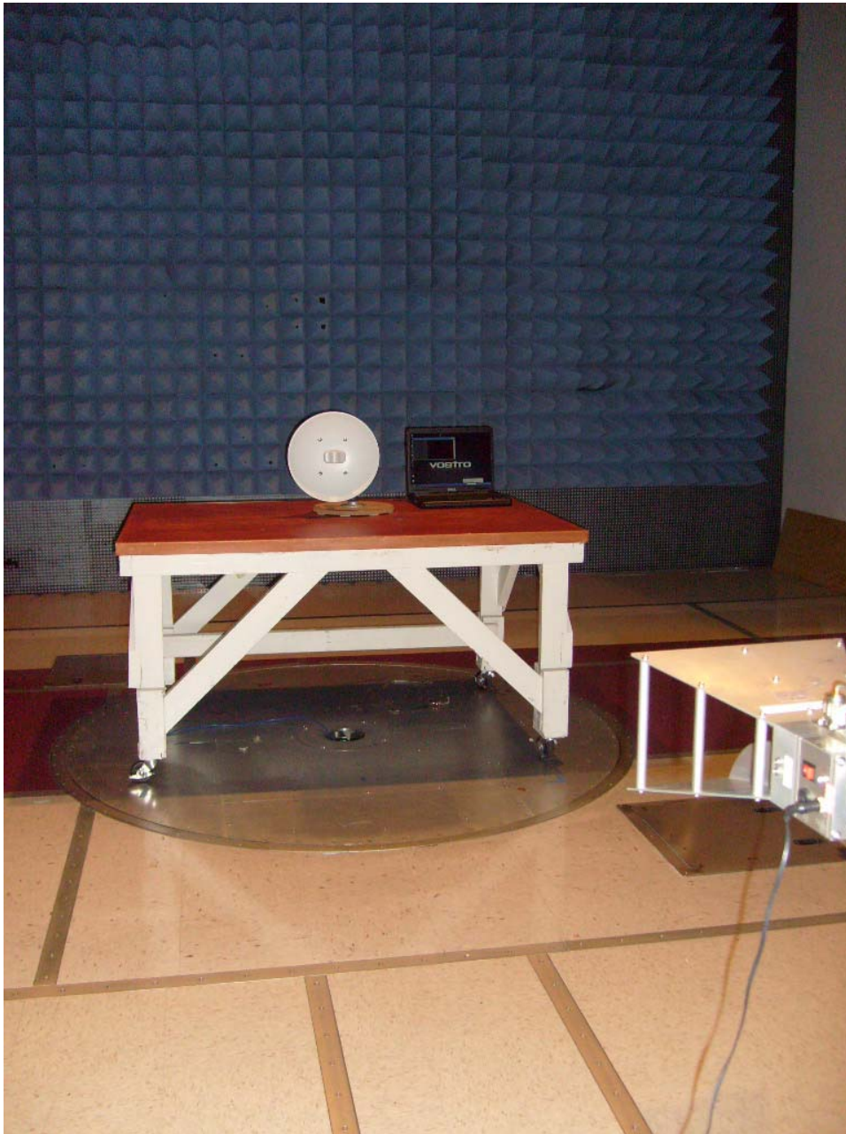
Photograph 3. Radiated Emission, above 1GHz Test Setup
