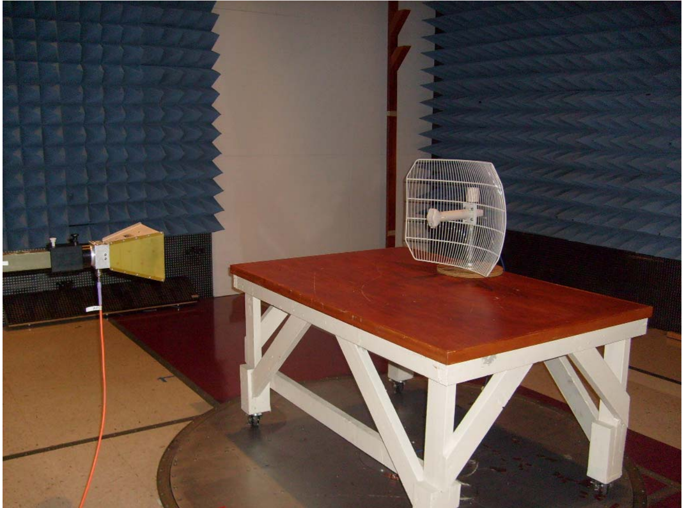
Photograph 6. Radiated Spurious, Test Setup (Grid Antenna)
