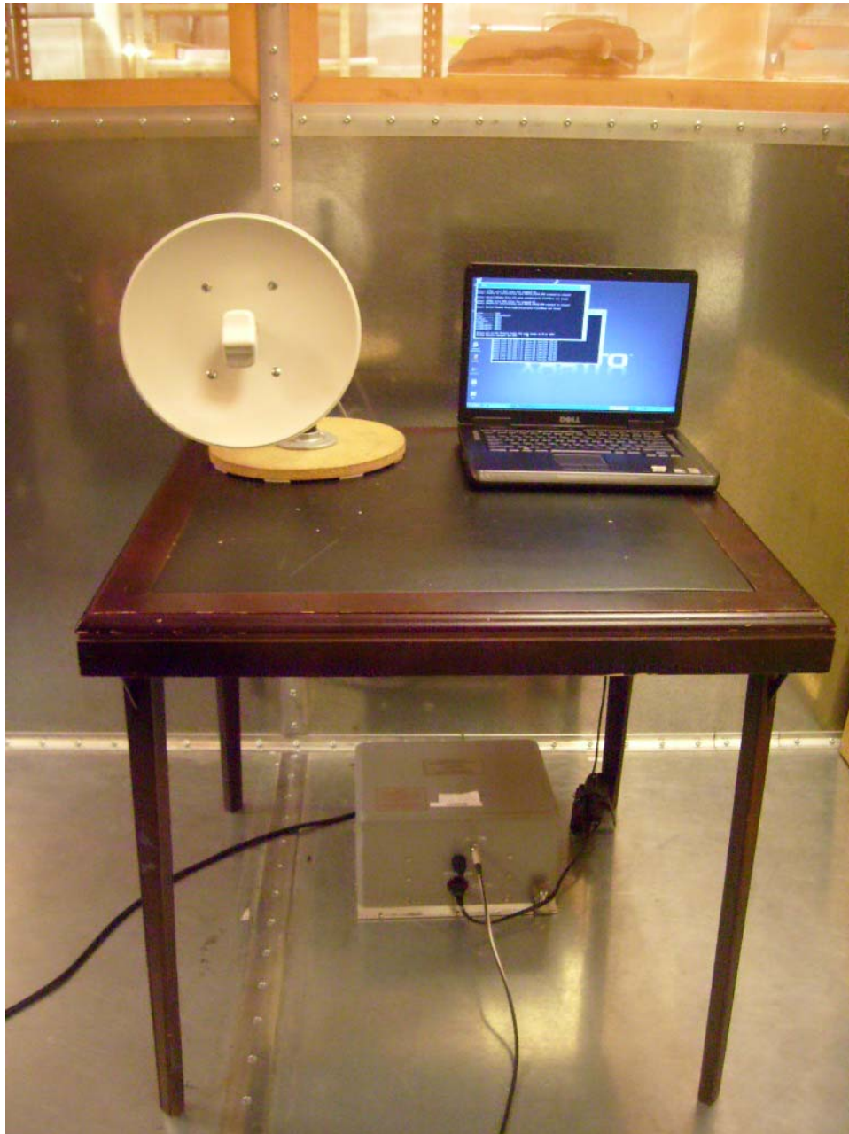
Photograph 1. Conducted Emissions, Test Setup
