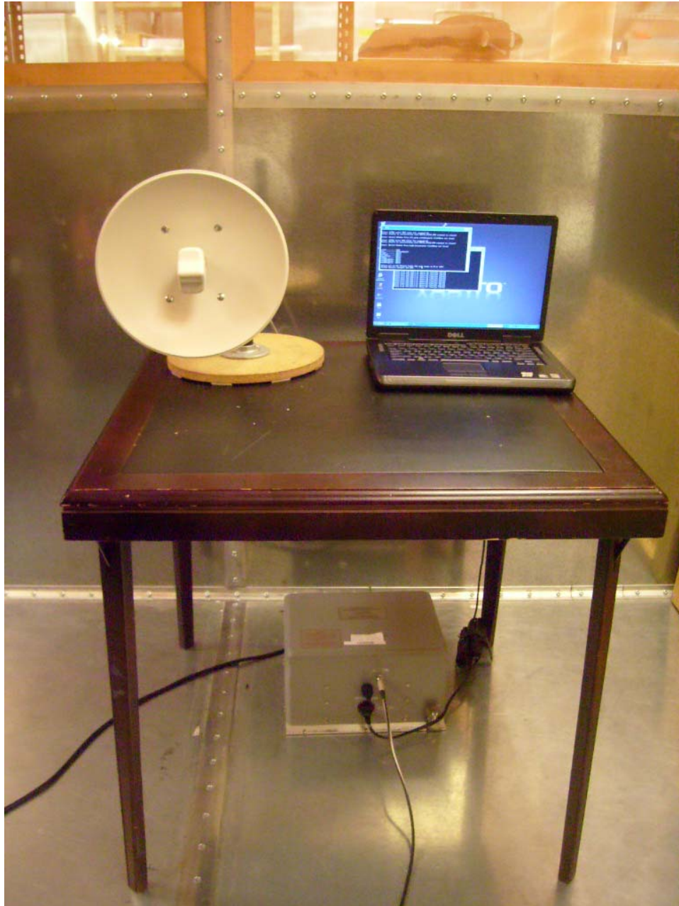
Photograph 4. Conducted Emissions, 15.207, Test Setup
