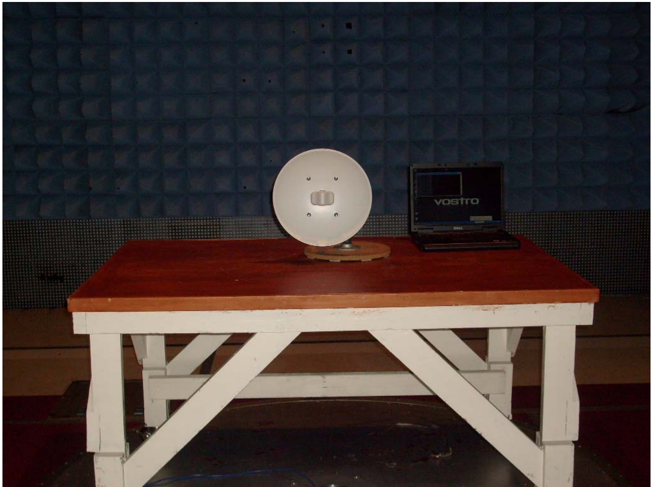
Photograph 2. Radiated Emission, Test Setup
