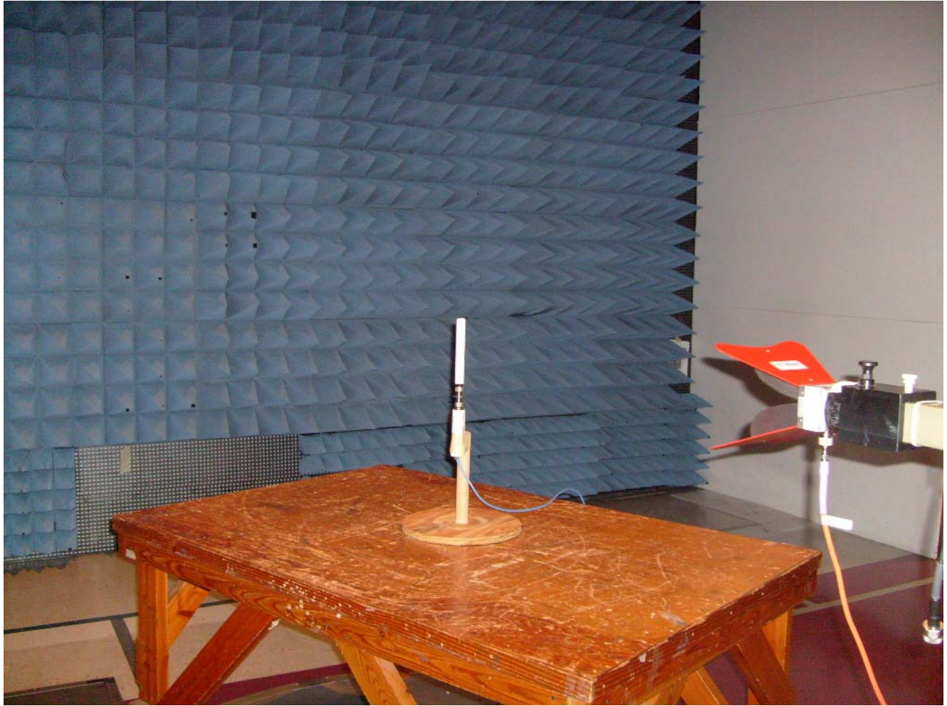
Photograph 6. Radiated Spurious Emission, Test Setup
