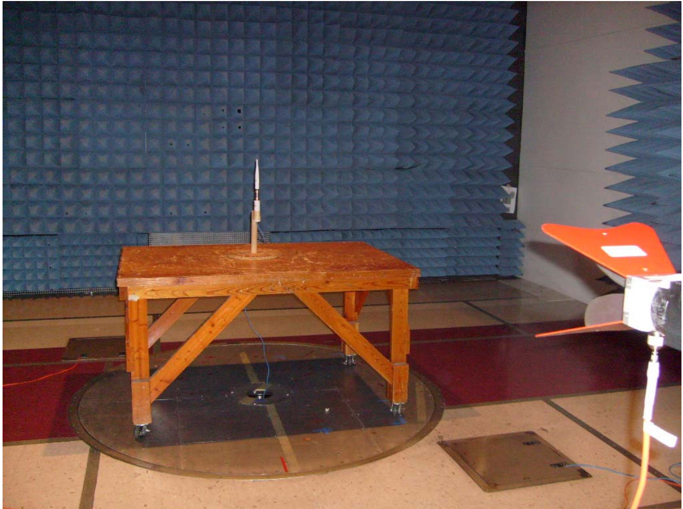
Photograph 7. Radiated Spurious Emission, Test Setup
