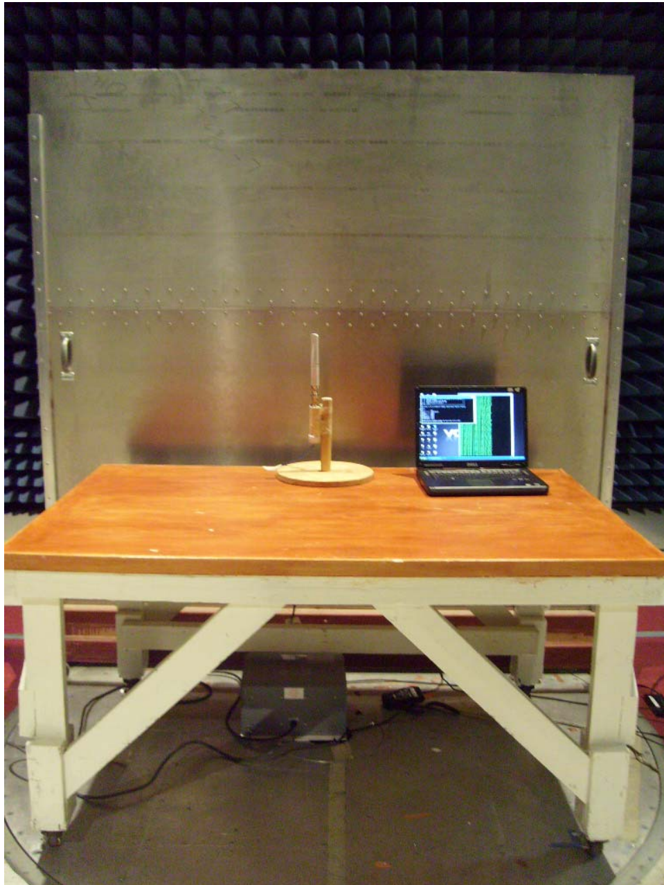
Photograph 1. Conducted Emissions, Test Setup
