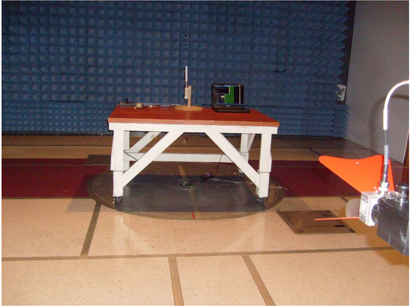
Photograph 3. Radiated Emission, above 1GHz Test Setup
