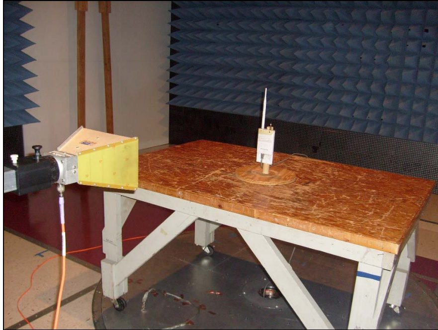
Photograph 6. Test Equipment and Setup for Various Radiated Measurements – Omni Antenna
