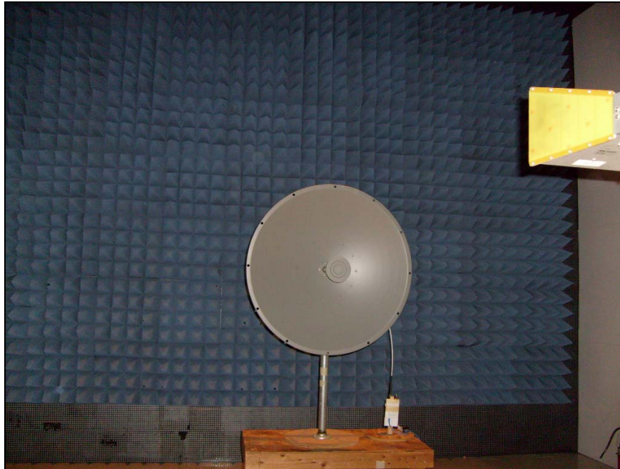
Photograph 8. Test Equipment and Setup for Various Radiated Measurements – Dish
