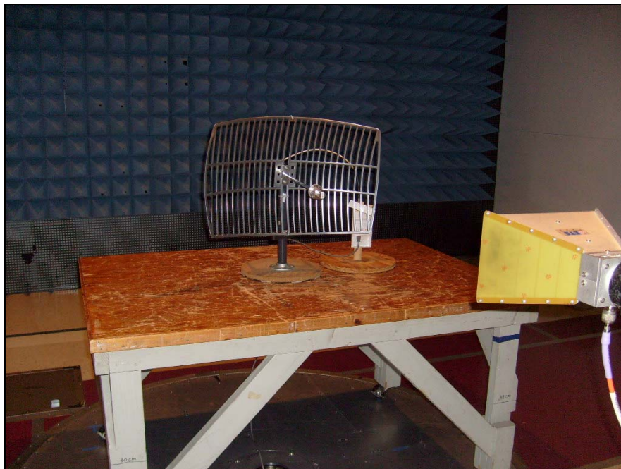
Photograph 9. Test Equipment and Setup for Various Radiated Measurements – Grid
