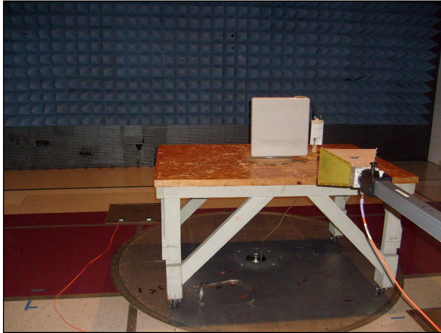
Photograph 10. Test Equipment and Setup for Various Radiated Measurements – Panel
