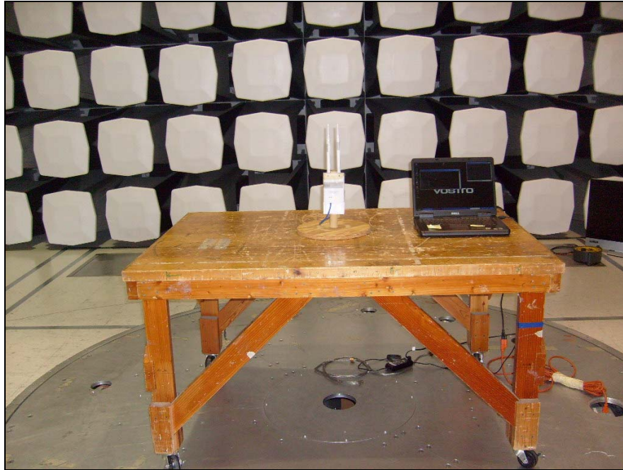
Photograph 3. Radiated Emission, Test Setup
