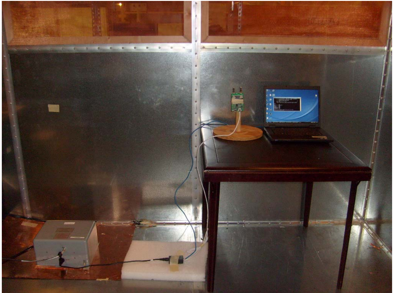
Photograph 2. Conducted Emissions Test Setup
