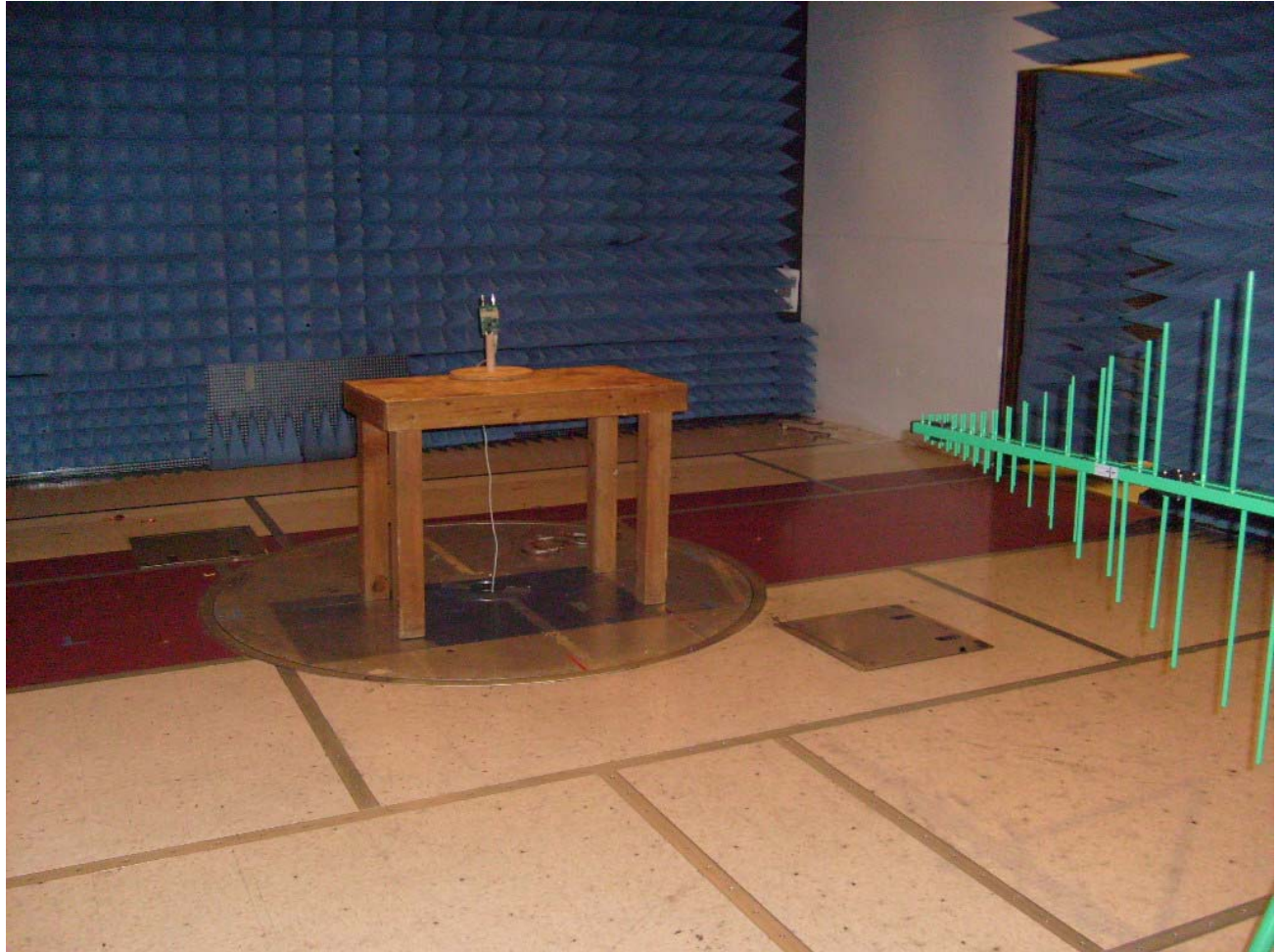
Photograph 6. Radiated Emission Spurious Bilog Antenna Test Setup
