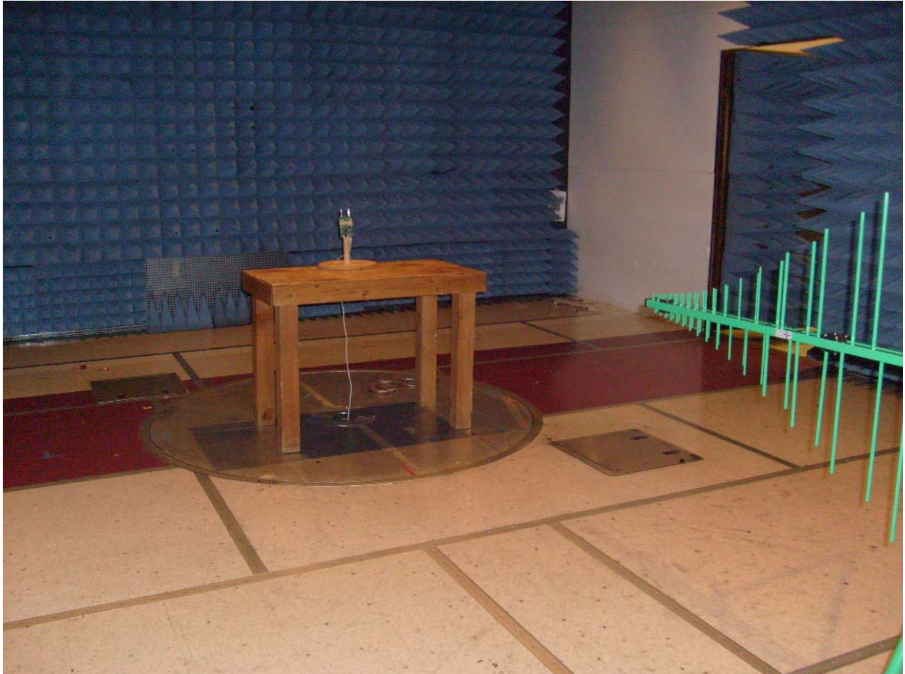
Photograph 3. Radiated Emission Limits 30MHz – 1GHz Test Setup
