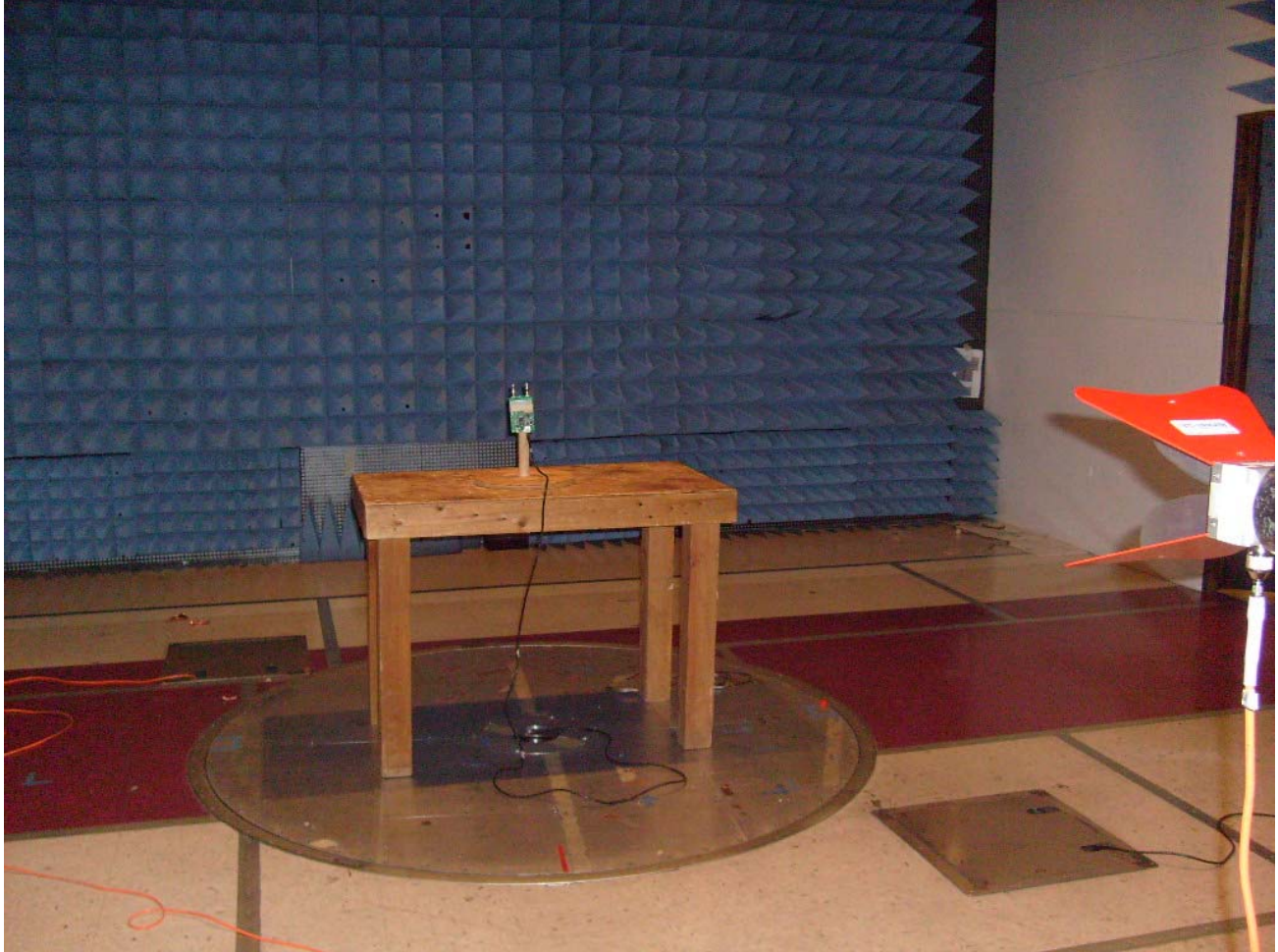
Photograph 7. Radiated Emission Spurious Horn Antenna Test Setup
