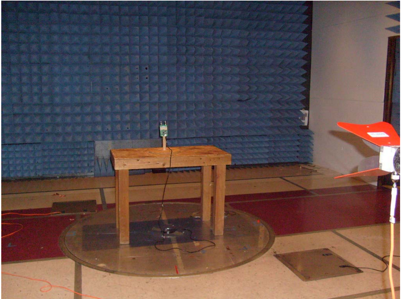
Photograph 4. Radiated Emission Limits 1GHz – 10GHz Test Setup
