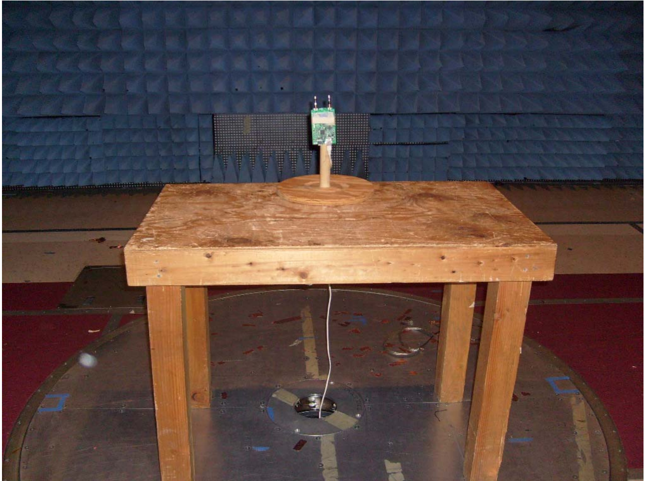
Photograph 5. Radiated Emission Spurious Test Setup
