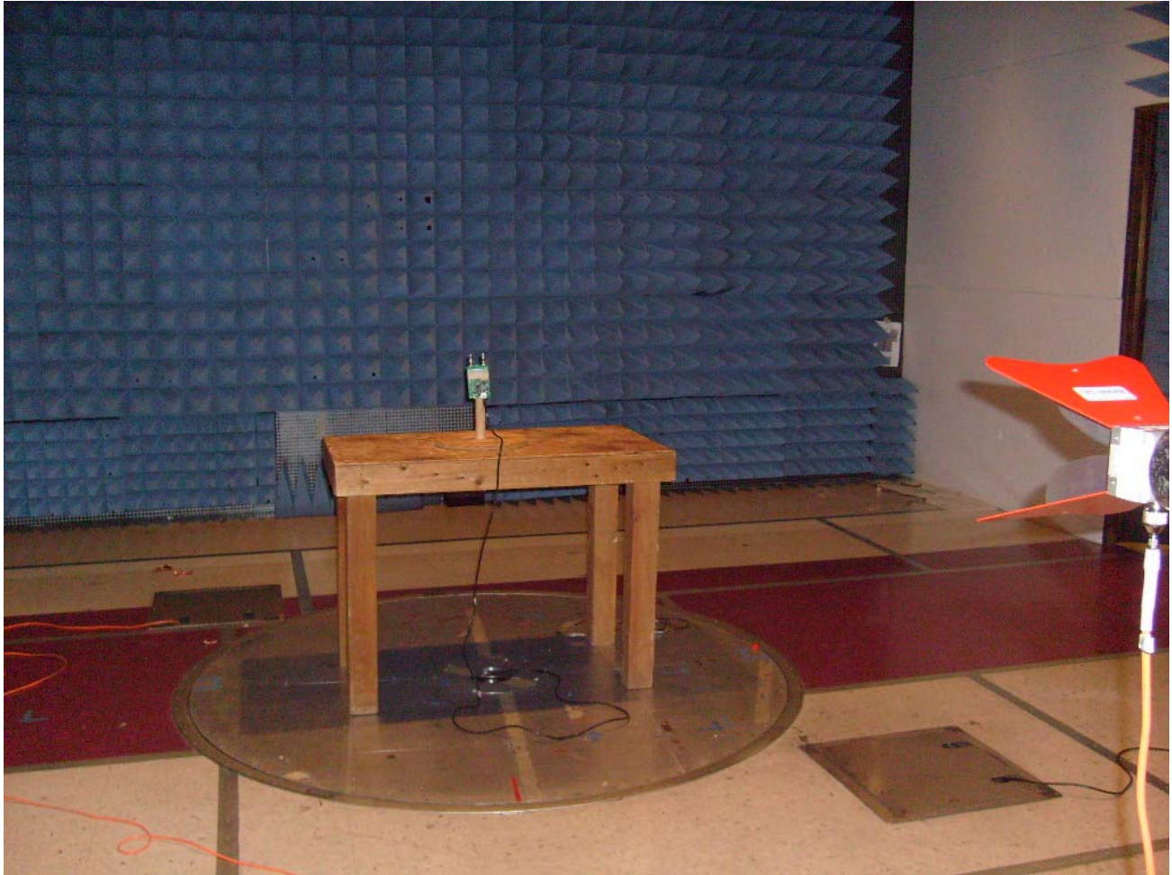
Photograph 7. Radiated Emission Spurious Horn Antenna Test Setup
