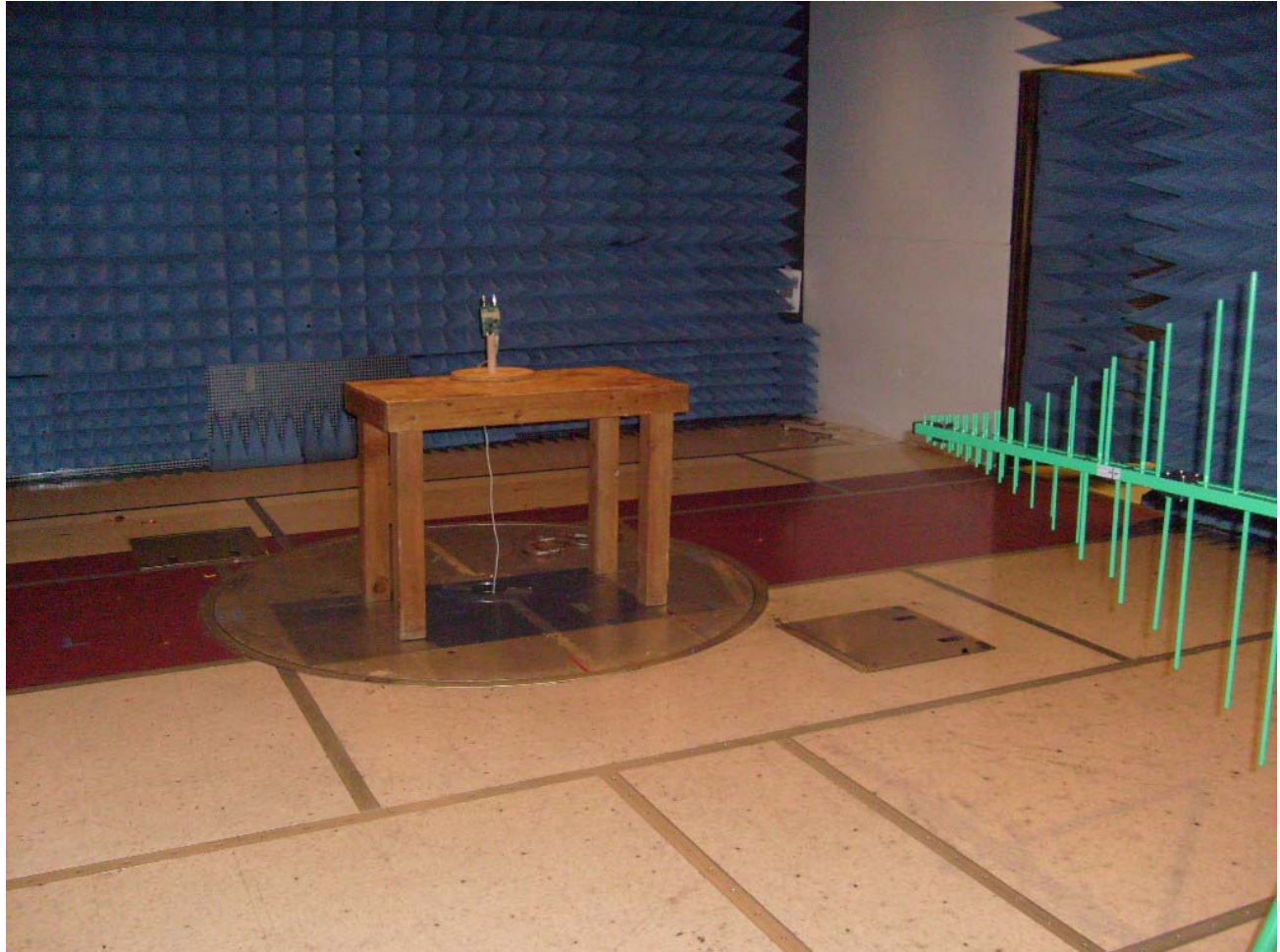
Photograph 6. Radiated Emission Spurious Bilog Antenna Test Setup
