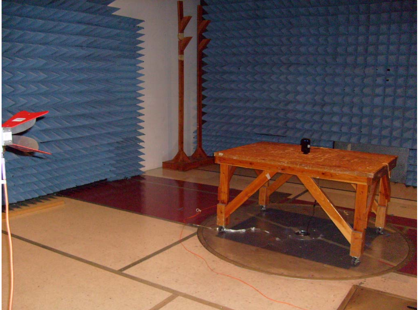
Photograph 6. Radiated Spurious Emissions, 3 meter Test Setup
