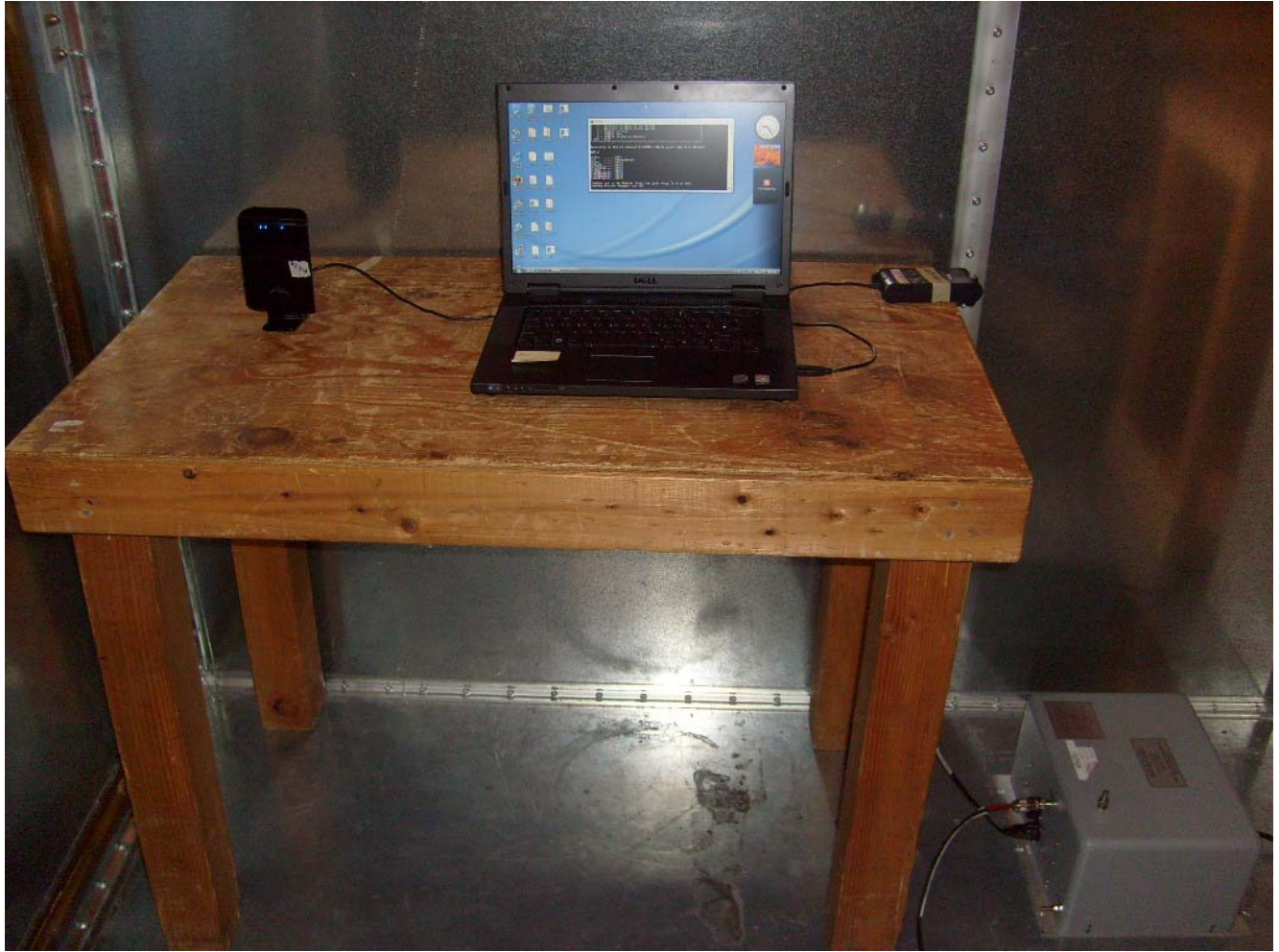
Photograph 2. Conducted Emissions, Test Setup
