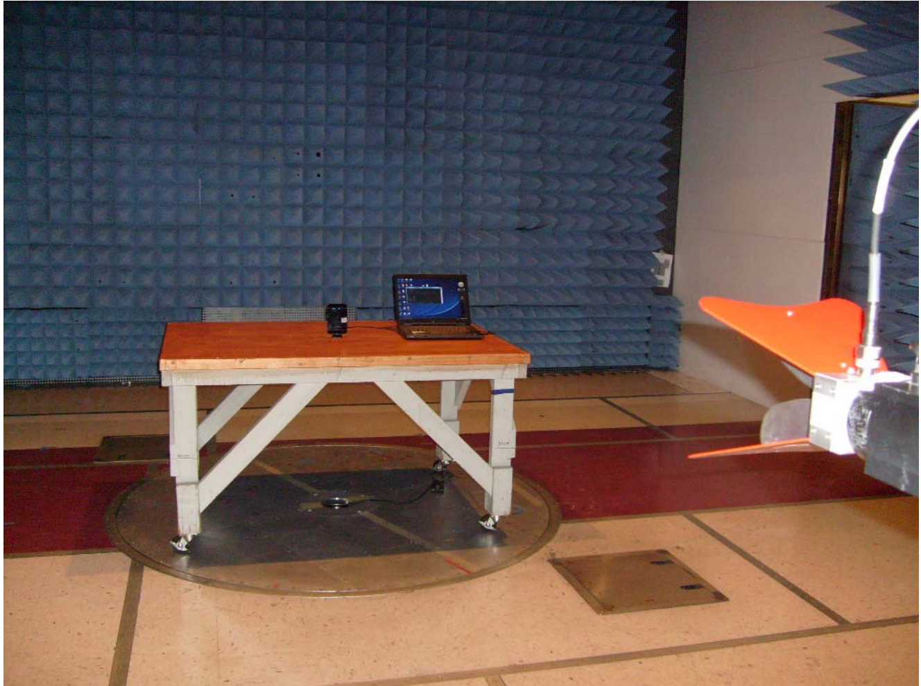
Photograph 4. Radiated Emission, Test Setup, above 1GHz
