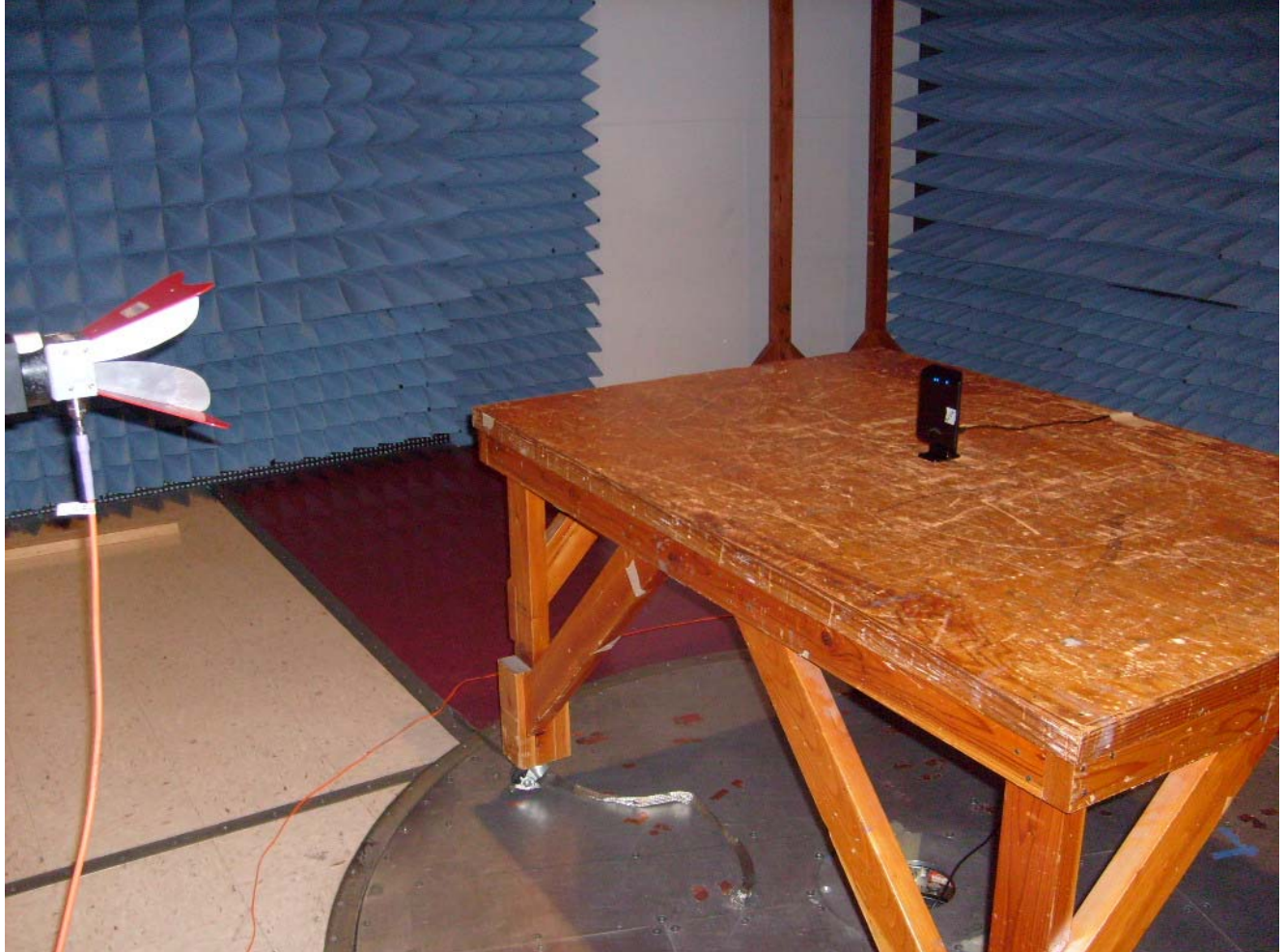
Photograph 7. Radiated Harmonics Emissions, 1 meter Test Setup
