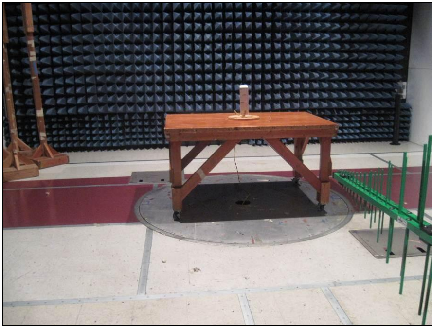
Photograph 8. Radiated Harmonic/Spurious Emissions, Test Setup, Bilog
