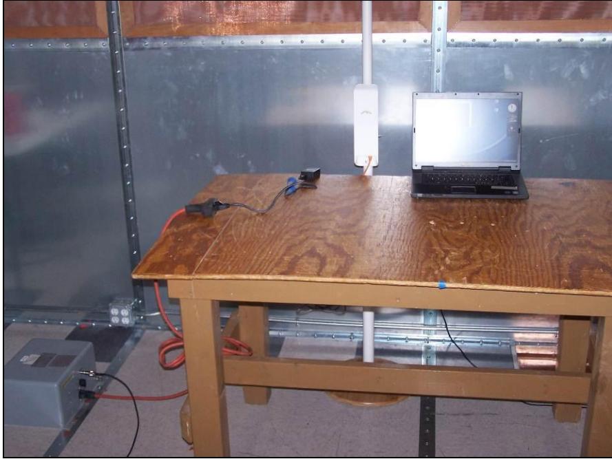
Photograph 1. Conducted Emissions, Test Setup, GME Power Supply
