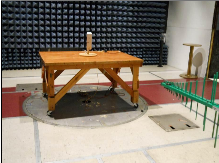
Photograph 4. Radiated Emission, Test Setup, Cetus Power Supply
