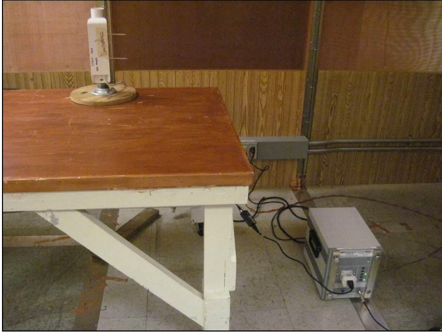
Photograph 5. Conducted Emissions, 15.207(a), Test Setup, GME Power Supply
