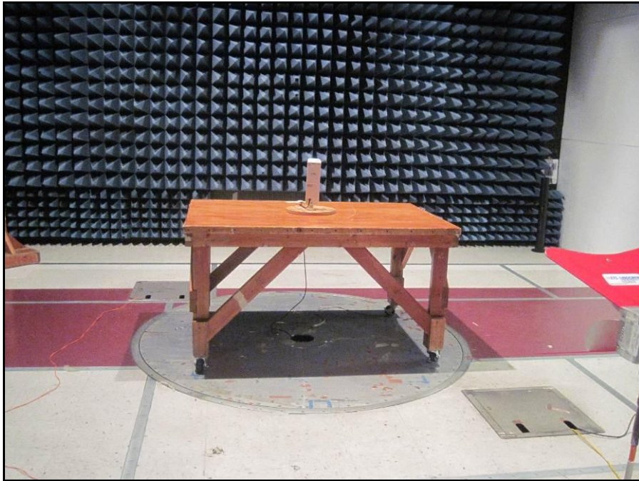
Photograph 10. Radiated Band Edge Emissions, Test Setup, 3m
