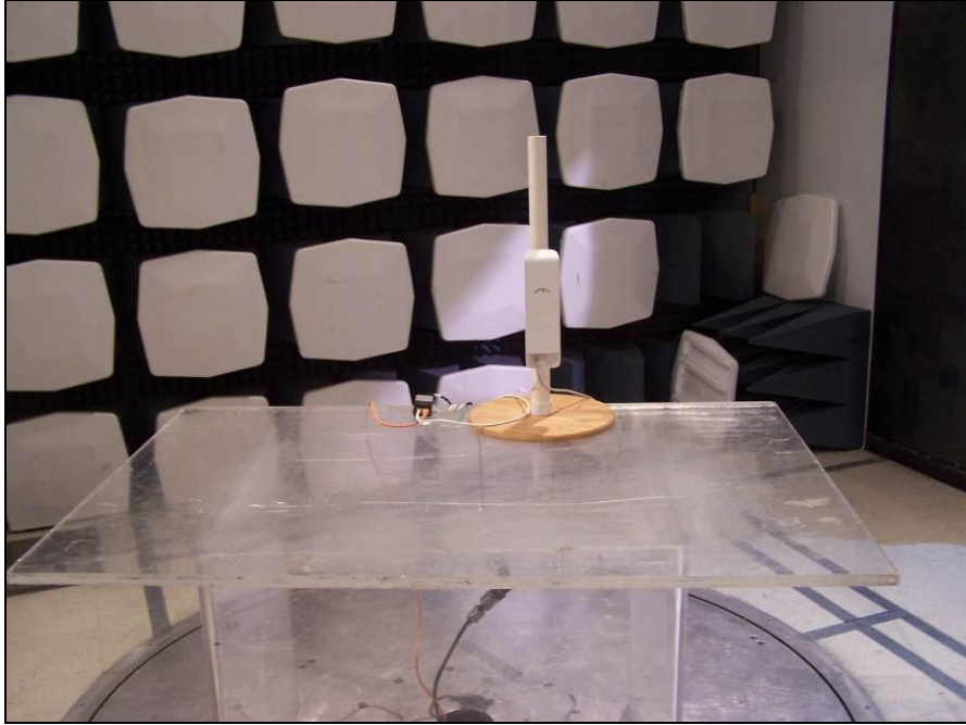
Photograph 3. Radiated Emission, Test Setup, GME Power Supply
