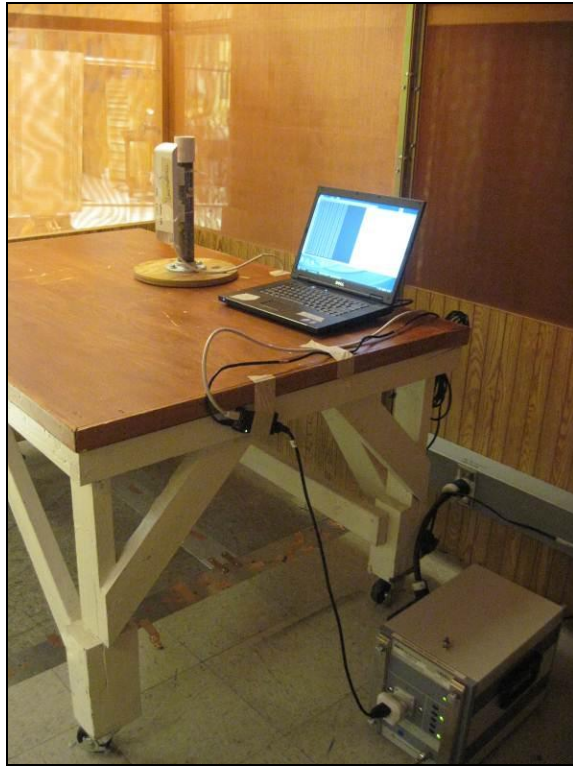
Photograph 2. Conducted Emissions, Test Setup, Cetus Power Supply
