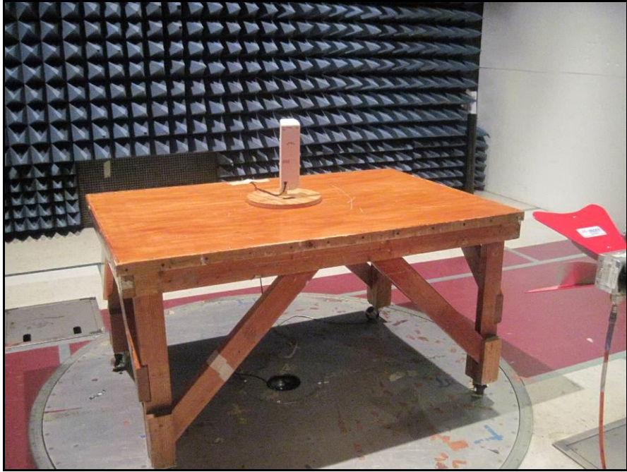
Photograph 7. Radiated Harmonic/Spurious Emissions, Test Setup, Horn
