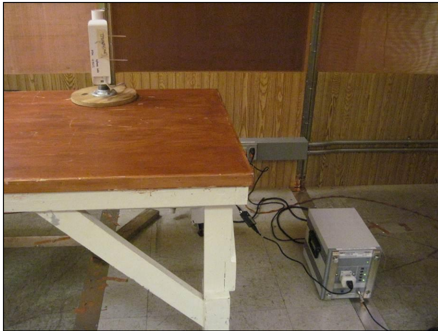
Photograph 6. Conducted Emissions, 15.207(a), Test Setup, GME Power Supply
